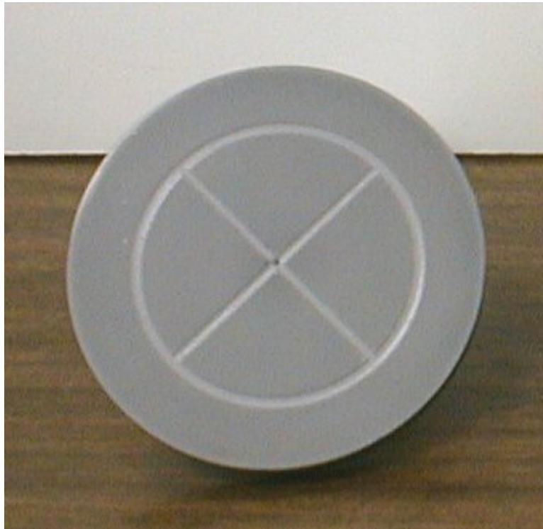
Figure 6.4. Fired glass-ceramic/molybdenum electrostatic chuck after polishing of the glass-ceramic (SCE-505) layer.
