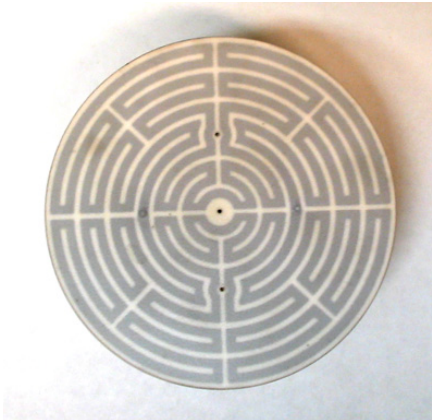
Figure 6.16. Ceramic plate heater with an alumina substrate, SCE-5 glass dielectric layers and Ag-Pd alloy for the resistor pattern.
