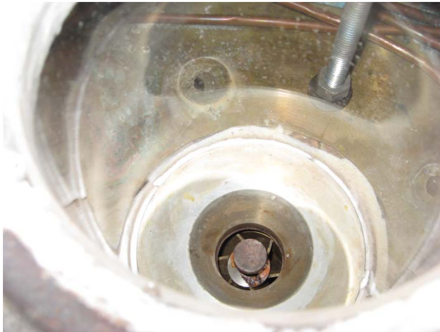
Figure 2.9 - Photograph of the swirl from the top of the quartz combustion section in which the centerbody and swirler are visible as installed for use.
