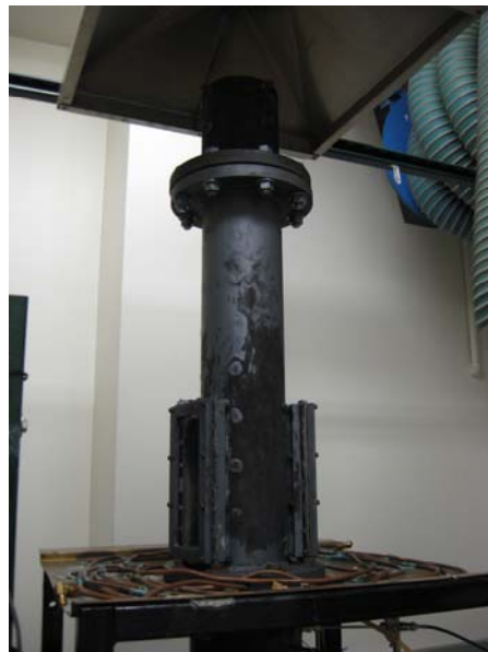
Figure 2.29 - Close up of the combustion section of the rig configured for self-excited operation.
