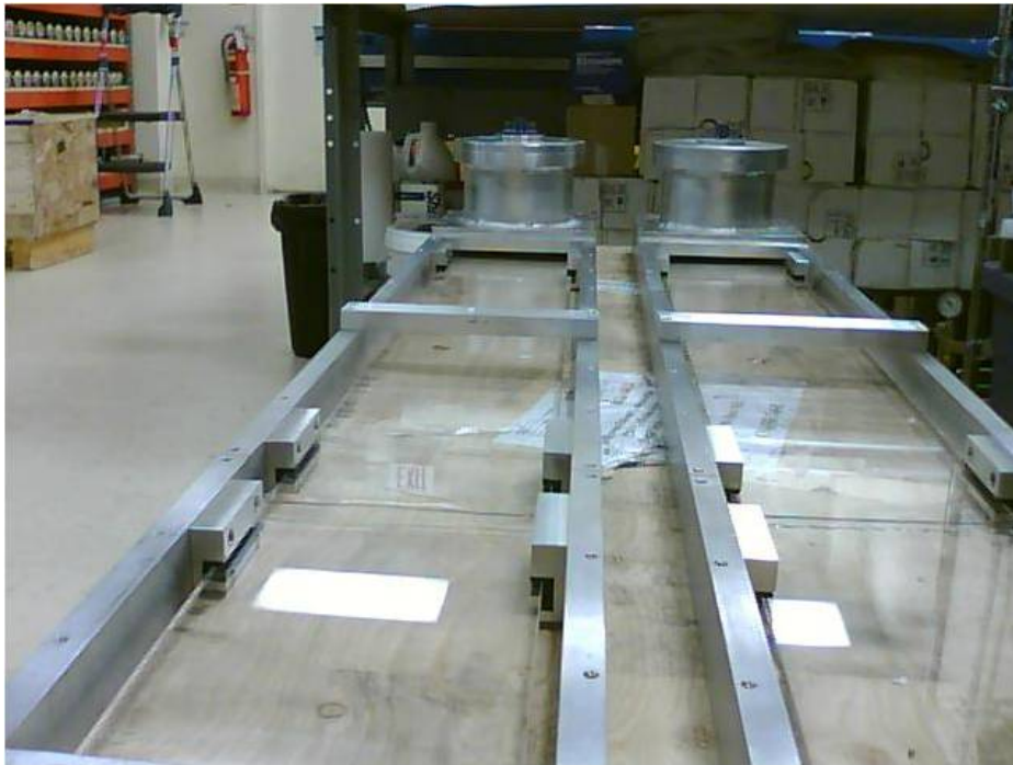
Figure 2.5: Photograph of two of the bars in the housing that will provide strain relief on the joint as well as structural support for the PMTs and the lead that will shield them[93].
