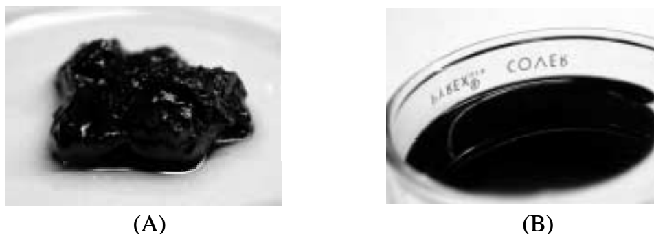
Figure 5.21 A cobalt dispersion prepared by using ethoxy-containing terpolymers in, (A) toluene, and (B) 2000 g/mol PDMS. The image (A) was taken after adding 2000g/mol PDMS and removing toluene.
