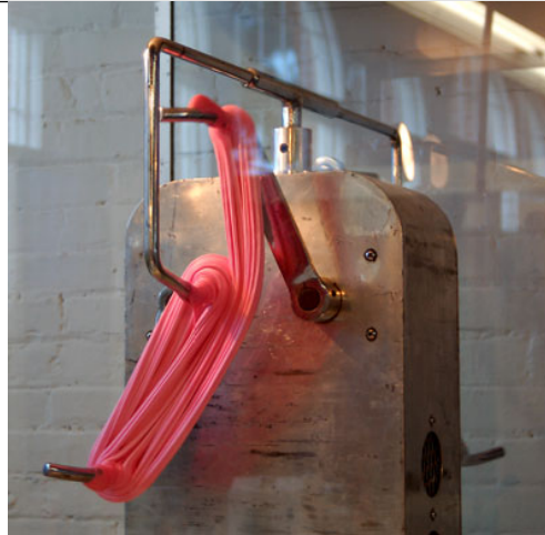
Figure 3.1: A three-rod taffy pulling mechanism. [picture by H. Greenside www.phy.duke.edu ]
