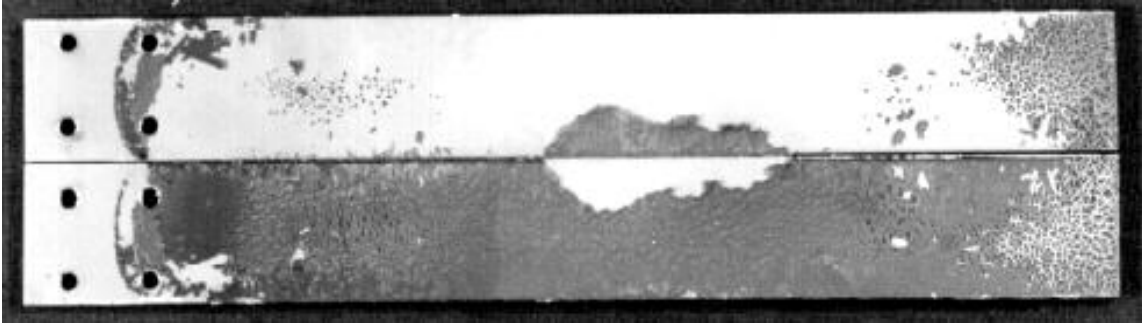
Figure 7.9 Photomicrograph of the fractured DCB specimen that was bonded for only two minutes.
