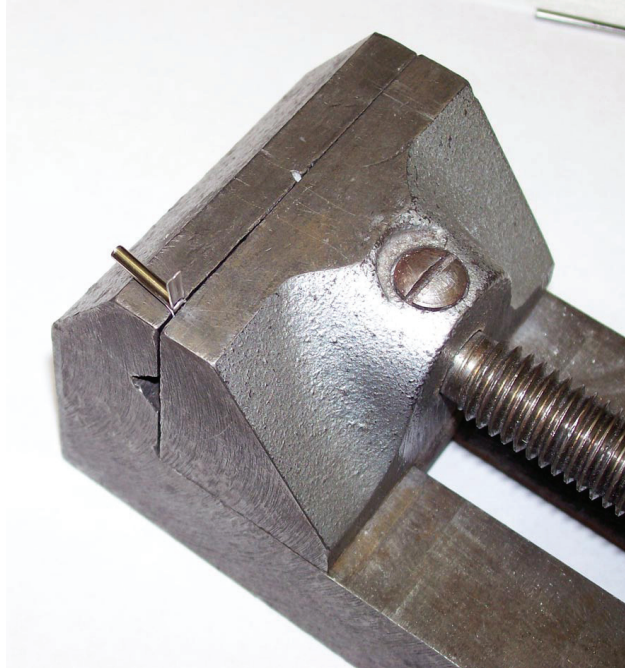
Figure A.10: Strain relief tube showing arms bent to 90° with vise.
