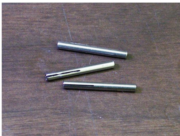
Figure A.8: Inconel strain relief tubes diced to length (0.75 in) with 0.375 in axial slot.
