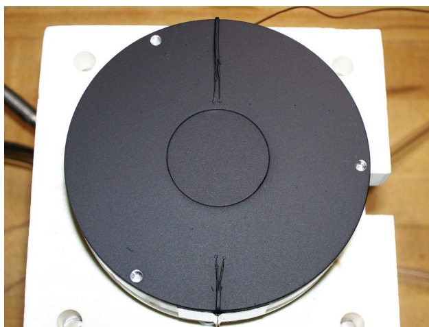
Figure B.6: Cold plate with Schmidt-Boelter reference sensor installed. The surface is coated first with two layers of Zynolyte (as shown), and then with one layer of GE Aerocoat carbon soot (not shown).
