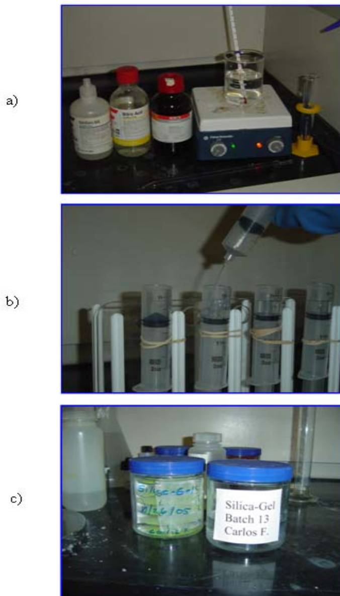
Fig. 4.1: Stages performed in Part I of the production process: a) precursor materials and mixing, b) casting and gelation, c) aging.
