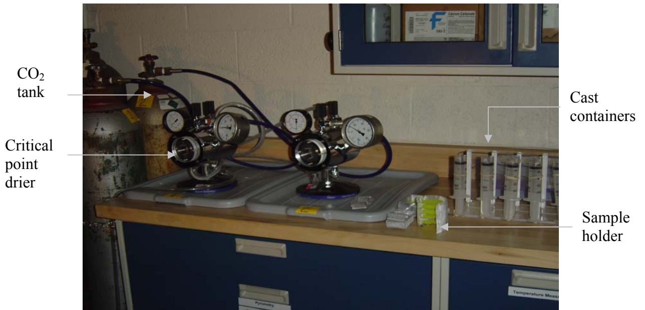
Fig. 4.3: Set-up used to make dried aerogel samples.
