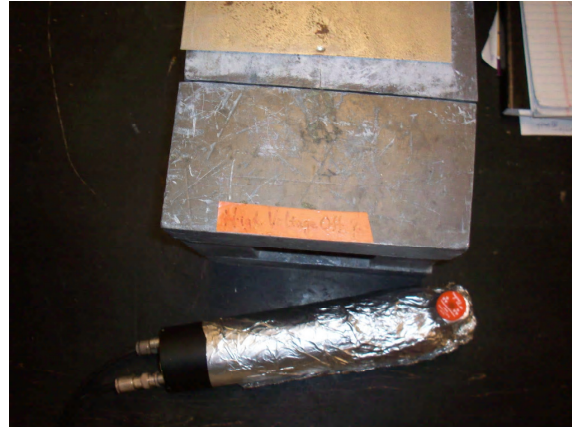
Figure 25 S% measurement system at VT. Lead housing, PMT with acrylic sample holder, and ^{137}\text{Cs} source.
