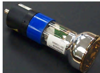
Figure 68 Photonis XP3300 PMT with base. This is the PMT model that will be used for miniLENS
