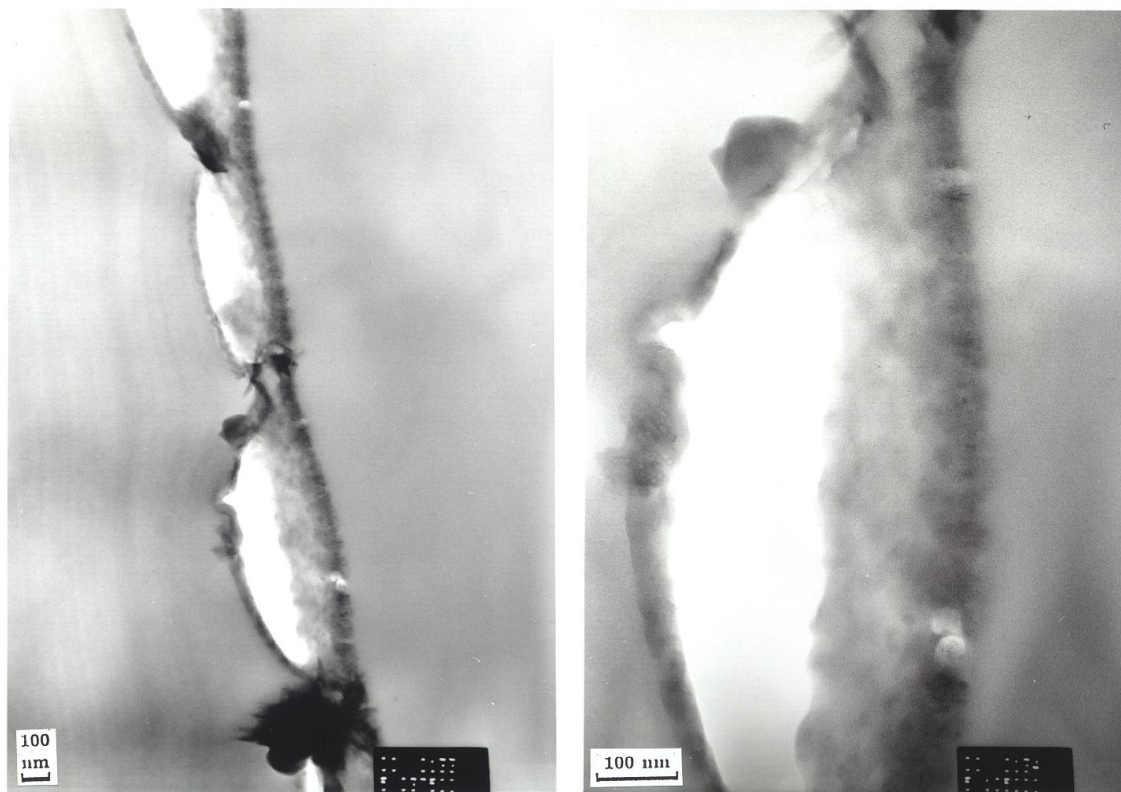
Figure 90 TEM images of a P3OT/C 60 bilayer heated at 130 °C. The image on the right is a magnification of the image on the left to better see the morphology. The film has come off the PES substrate in most areas, but TEM images of the film could still be taken. The images show that the interface between P3OT and C 60 has become rougher than in the unheated bilayer and clusters of C 60 have moved into the film.
