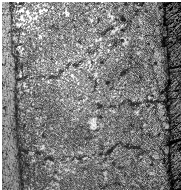
Figure 34. Longitudinal matrix cracking in virgin specimen
