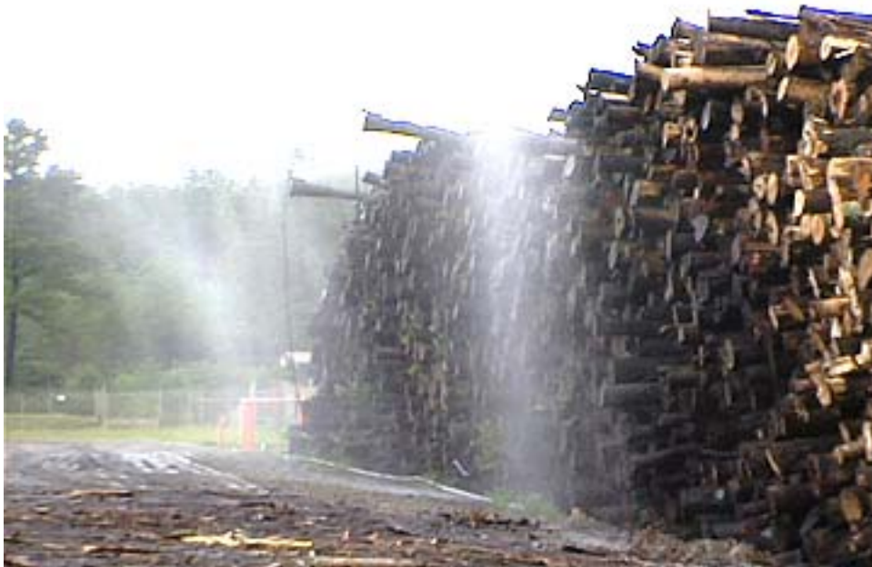
Figure II.9. Wood is stored under sprinklers to extend its useful life.
