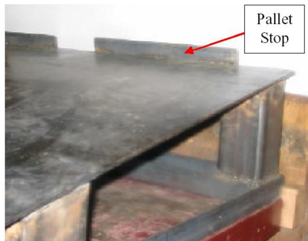
Figure 89 Photograph of the Pallet Stop fabricated into the steel leveling table
