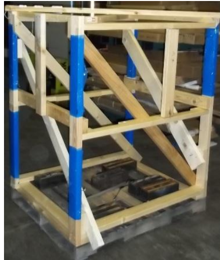
Figure 13 Test frame used to simulate a unit load
