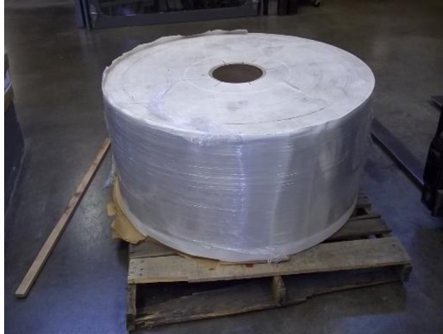
Figure 64 Round unit load recommended for wrapping during prestretching evaluation
