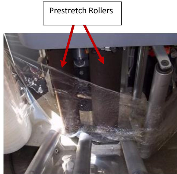
Figure 4 Where prestretching occurs in the application process
