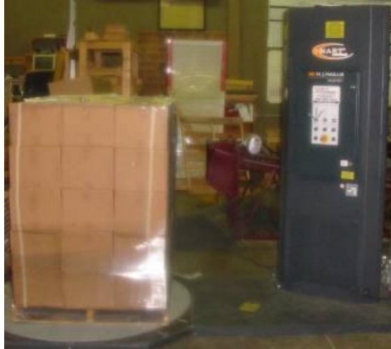
Figure 86 Photograph of the Wulftech Stretch Wrap Machine used to Apply
