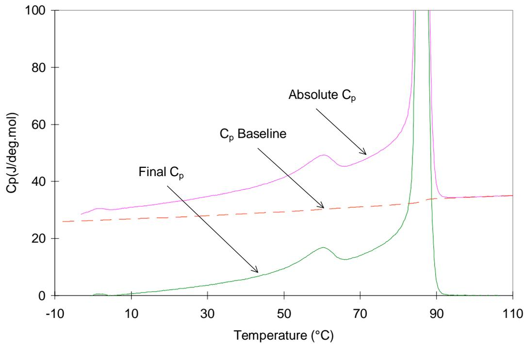
Figure 2 Absolute heat capacities, the  $C_p$  baseline and the "final" heat capacities for EB-912 cooled from the melt at  $20^\circ\text{C}/\text{min}$ .
