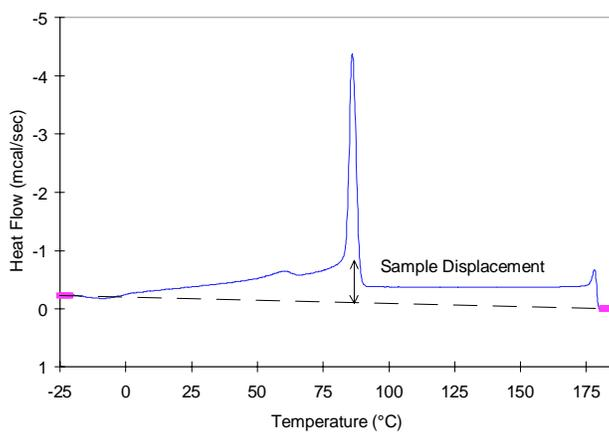
Figure 1 The displacements corresponding to the baseline, sapphire and the copolymer, EB-912 during cooling from the melt (180°C) at 20°C/min.
