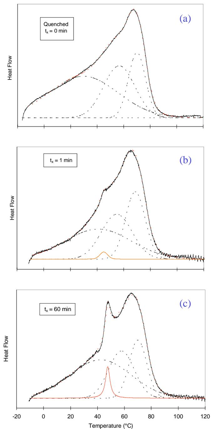
Figure 3 Evolution of the low endotherm for EB-883 quenched from the melt (160°C) to -20°C and subsequently crystallized at  $T_x = 40^\circ\text{C}$  for various times. The Gaussian peaks used in the deconvolution are also shown (black lines). The red curve represents the low endotherm. (a) Quenched, (b)  $t_x = 1$  min, (c)  $t_x = 60$  min.
