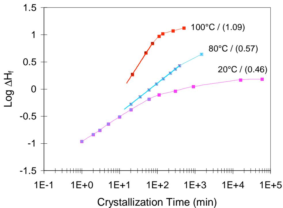
Figure 21 Avrami plots for EB-912 (with ~ 5 mole % butene) crystallized at various temperatures. The numbers indicate  $T_x/(n)$ .
