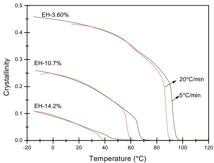
Figure 7 Degrees of crystallinity as a function of temperature obtained at different cooling rates from the melt for ethylene/1-hexene copolymers of various branch contents
