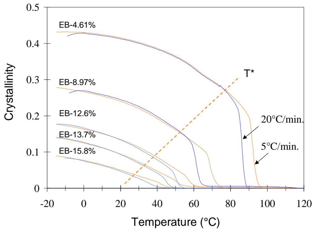
Figure 5 Degrees of crystallinity as a function of temperature obtained at different cooling rates from the melt for ethylene/1-butene copolymers of various branch contents
