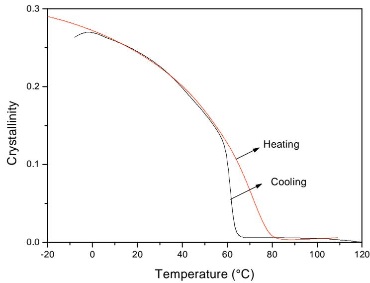
Figure 8 Degrees of crystallinity as a function of temperature for EB-894 during cooling at 20°C/min from the melt and during subsequent heating at 20°C/min.
