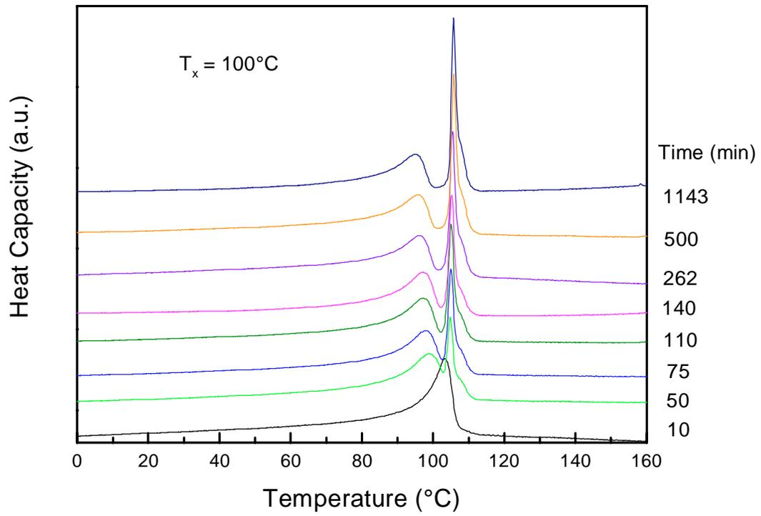
Figure 19 DSC thermograms for EB-912 after crystallization for various times at 100°C
