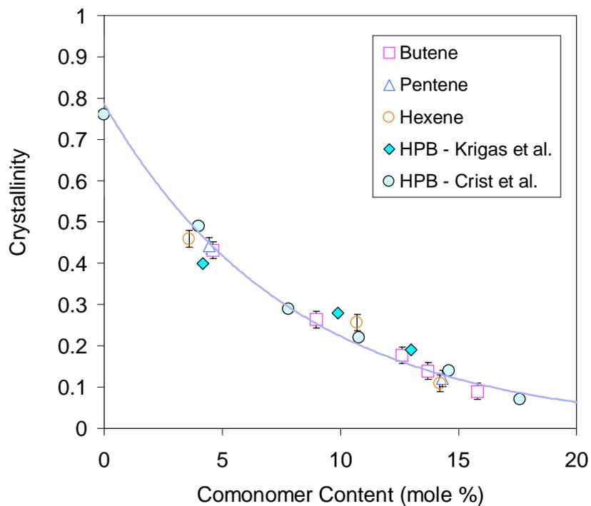
Figure 1 Degrees of crystallinity at  $-20^{\circ}\text{C}$  for ethylene/1-butene, ethylene/1-pentene and ethylene/1-hexene copolymers (after cooling from the melt at  $5^{\circ}\text{C}/\text{min}$ ) as a function of comonomer content. The crystallinity data for HPBs<sup>6,7</sup> are also included.
