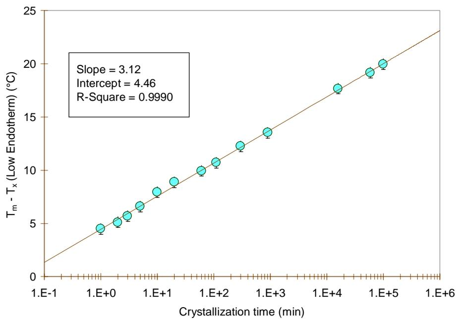
Figure 11 Relative positions of the low endotherms for EB-912 after crystallization for various times at 20°C
