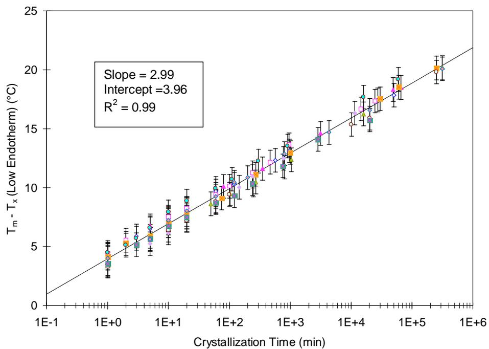
Figure 15 Relative positions of the low endotherms for ethylene/1-butene, ethylene/1-pentene and ethylene/1-hexene copolymers after crystallization for various times at  $20^{\circ}\text{C}$
