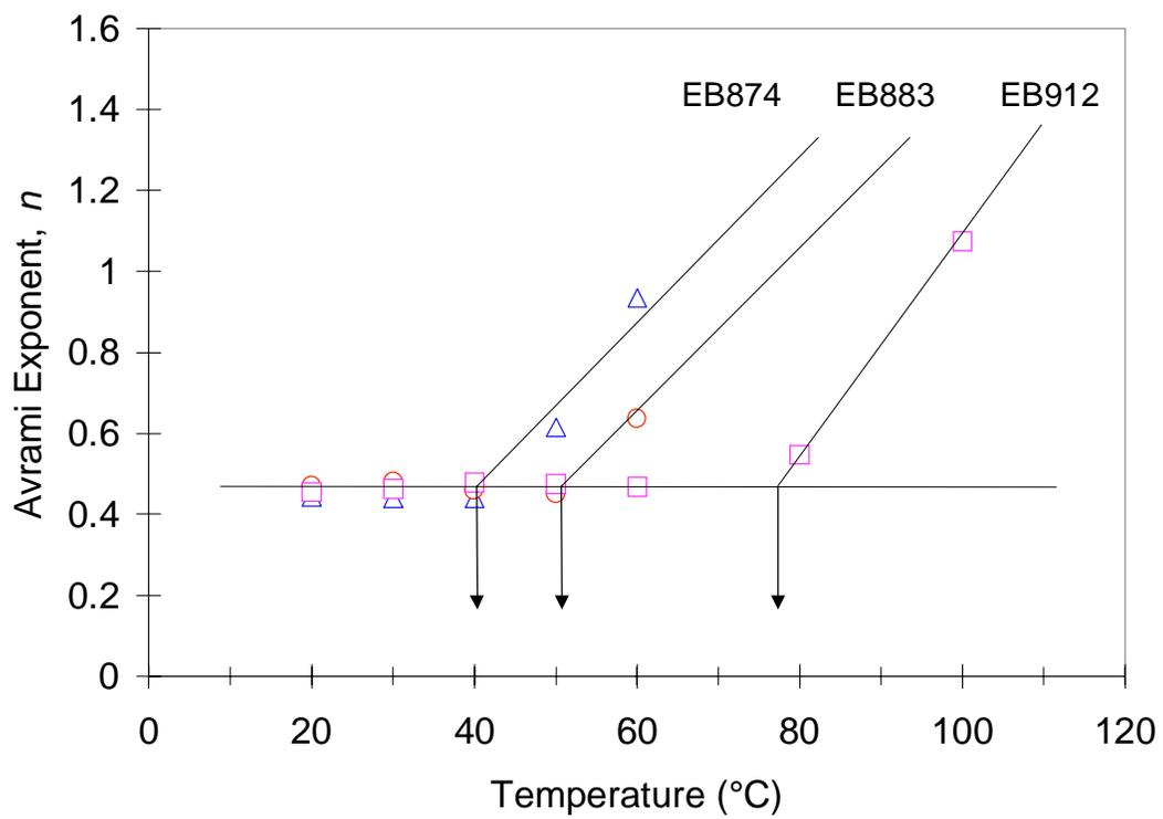
Figure 24 Avrami exponents,  $n$ , as a function of crystallization temperature for the ethylene/1-butene copolymers of various branch contents
