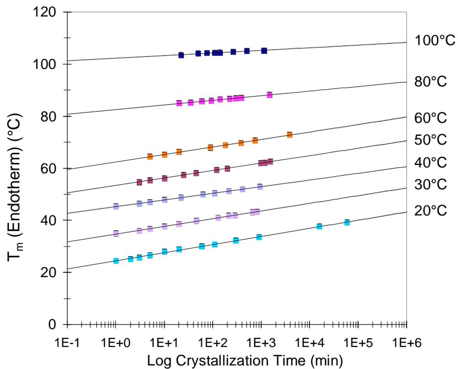
Figure 20 Peak positions of the endotherms for EB-912 after crystallization at various times for  $T_x$  ranging from 20 to 100°C
