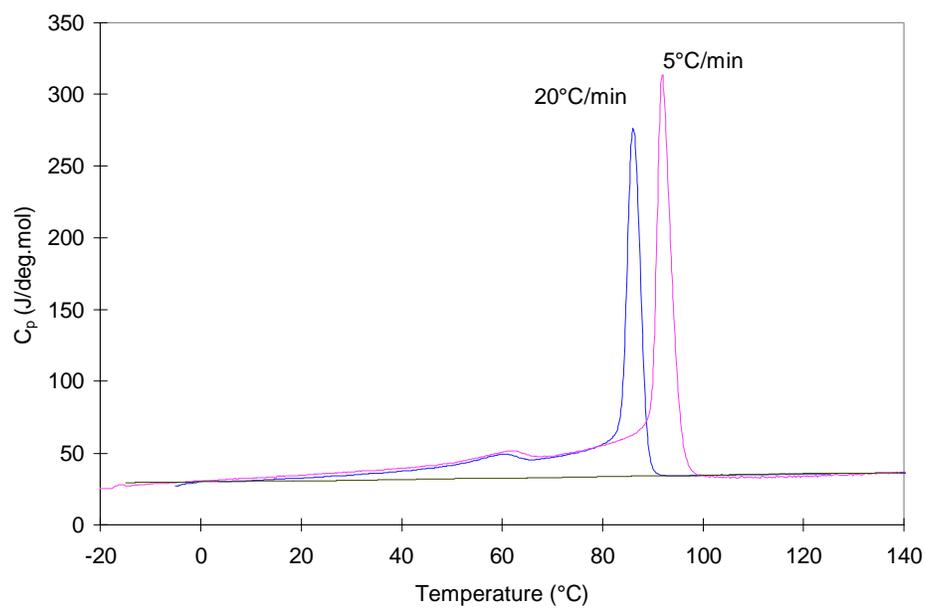
Figure 3 Corrected heat capacities for EB-912 during cooling from the melt at different rates
