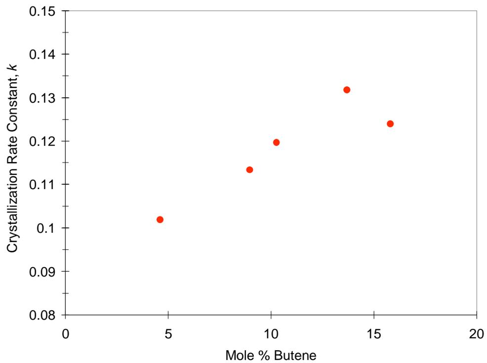
Figure 17 Crystallization rate constant,  $k$  as a function of branch concentration for ethylene/1-butene copolymers
