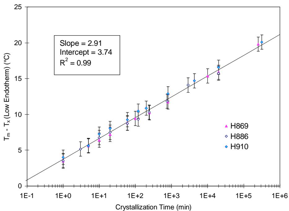
Figure 14 Relative positions of the low endotherms for ethylene/1-hexene copolymers after crystallization for various times at 20°C
