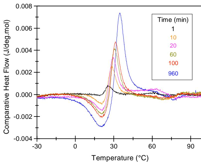
Figure 10 Curves obtained by subtraction of heating traces after finite crystallization times at 20°C from that of the quenched sample for EB-883
