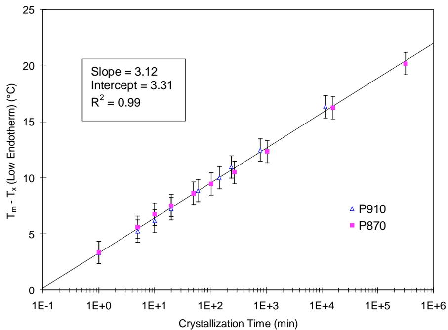
Figure 13 Relative positions of the low endotherms for ethylene/1-pentene copolymers after crystallization for various times at  $20^{\circ}\text{C}$
