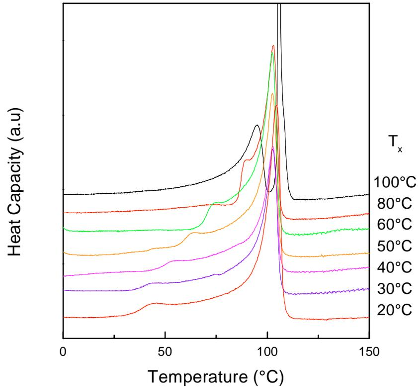
Figure 18 DSC thermograms for EB-912 after crystallization for long times at different crystallization temperatures
