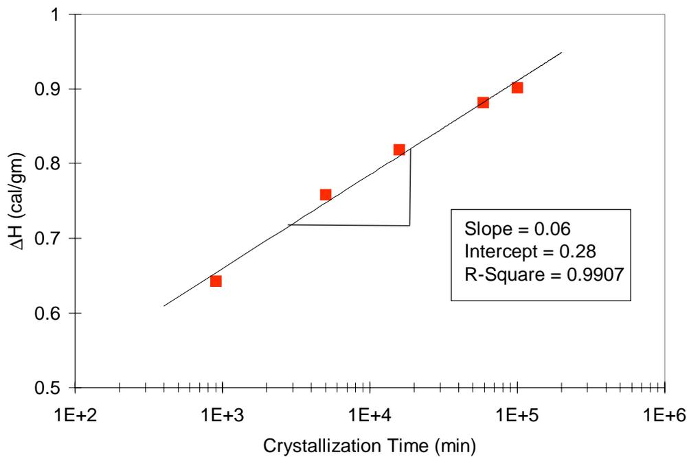
Figure 16 Typical Avrami plot for EB-912 after crystallization for various times at 20°C. The parameters corresponding to short (top) and long (bottom) times are also indicated
