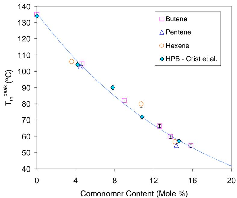
Figure 2 Peak melting temperatures for ethylene/1-butene, ethylene/1-pentene and ethylene/1-hexene copolymers as a function of comonomer content. The peak melting temperatures for HPBs<sup>7</sup> are also included.
