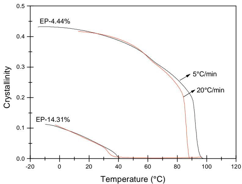
Figure 6 Degrees of crystallinity as a function of temperature obtained at different cooling rates from the melt for ethylene/1-pentene copolymers of various branch contents
