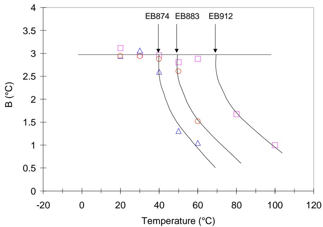
Figure 23 Variation of  $B$  as a function of crystallization temperature for the ethylene/1-butene copolymers of various branch contents
