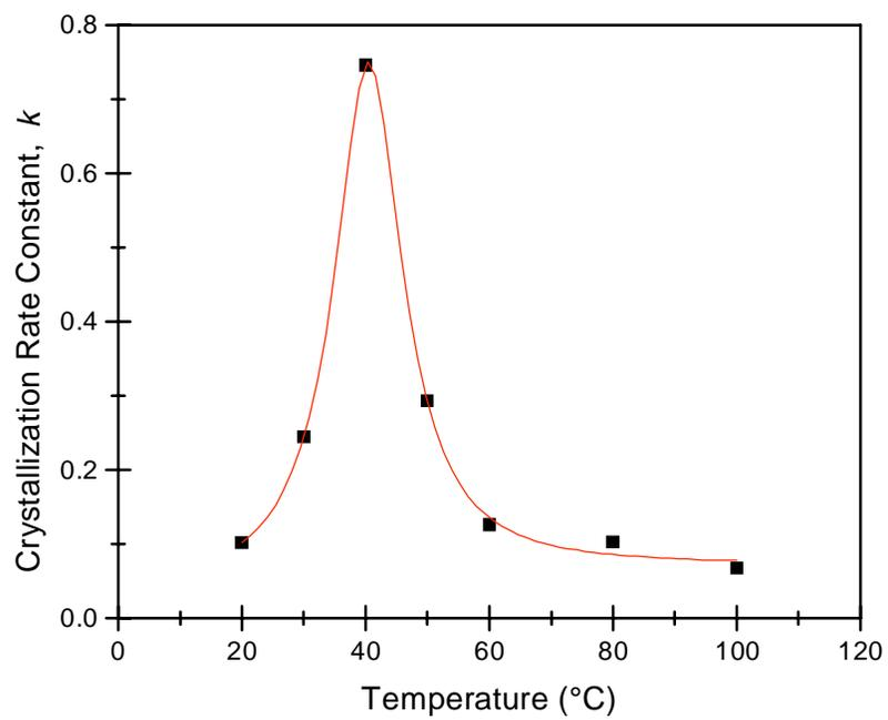
Figure 22 Normalized rate constant,  $k$ , for EB-912 as a function of crystallization temperature
