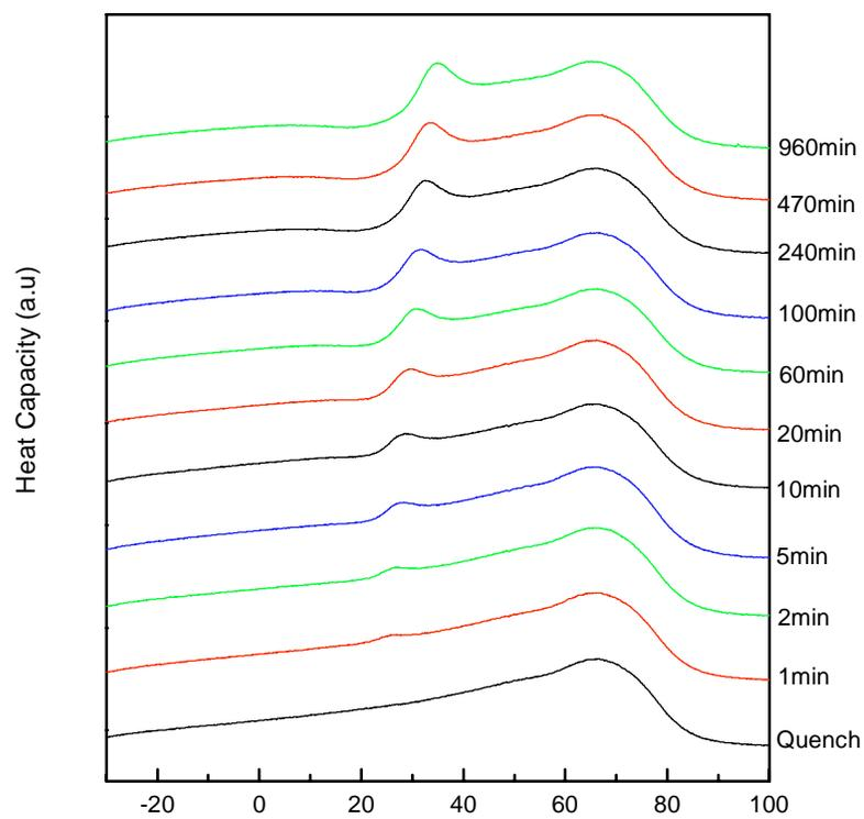
Figure 9 DSC thermograms for EB-883 after crystallization for various times at 20°C
