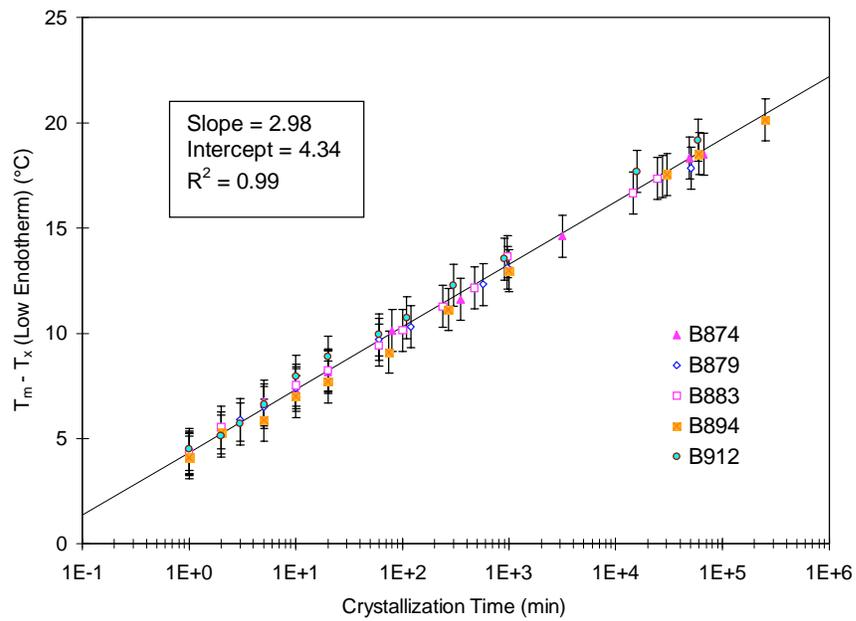
Figure 12 Relative positions of the low endotherms for ethylene/1-butene copolymers after crystallization for various times at  $20^{\circ}\text{C}$
