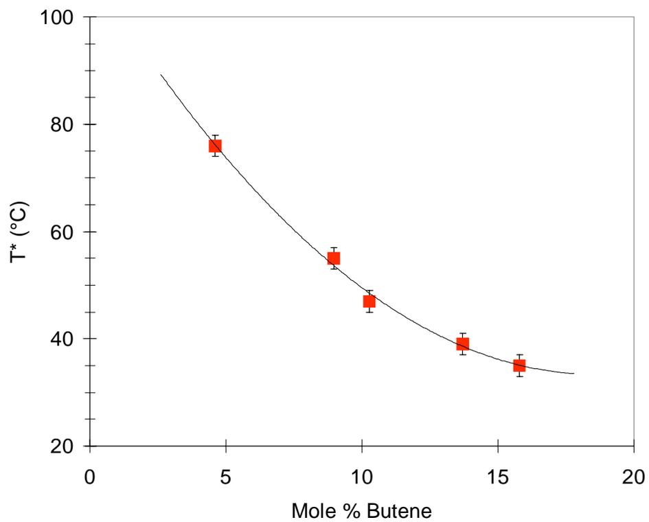
Figure 25 Variation of the cross-over temperature,  $T^*$ , with comonomer content for the ethylene/1-butene copolymers
