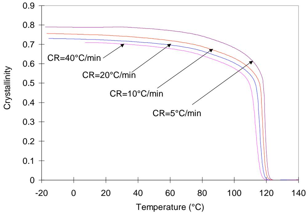
Figure 4 Degrees of crystallinity as a function of temperature obtained at different cooling rates from the melt for linear polyethylene (from Dr. A. Alizadeh)
