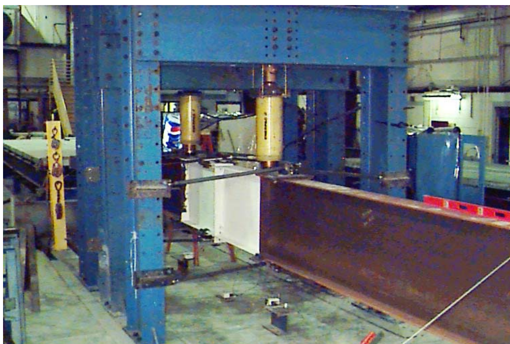
FIGURE 3.18: PHOTOGRAPH OF A MONOTONIC TEST SETUP
