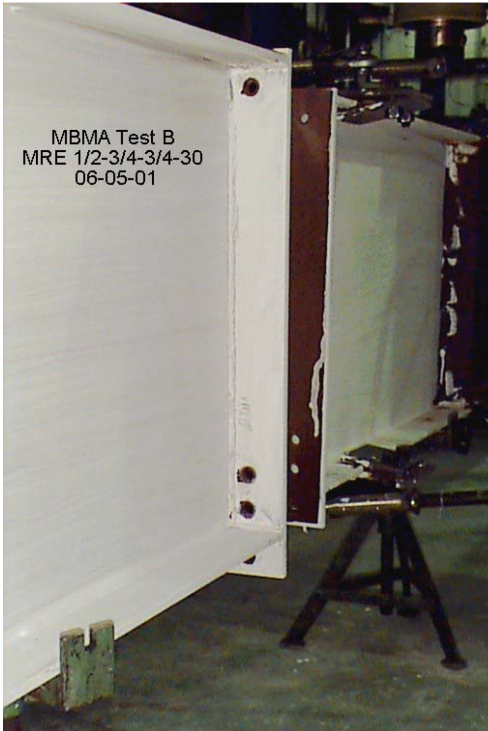
FIGURE 3.27: PHOTOGRAPH OF THICK PLATE FAILURE (TEST B - MRE 1/2-3/4-3/4-30)
