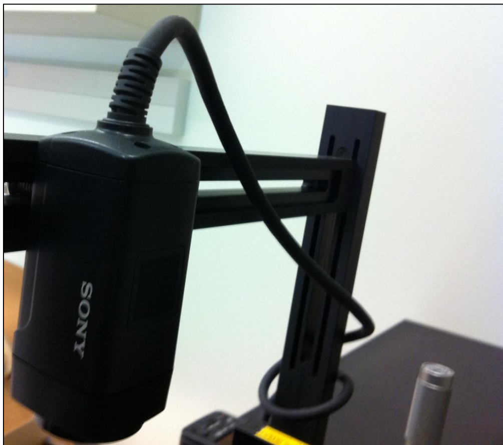
Figure 3.12. Top: Micropositioner is shown. The “L” shape extension can be seen at the top. Bottom: The camera mounted to the camera shaft.
