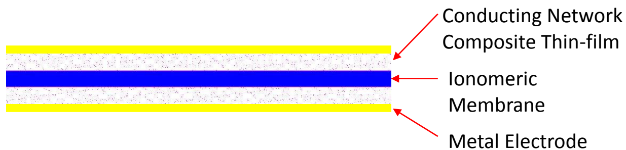
Figure 2.1. A not-to-scale schematic of a five layer IEAP bending actuator. Ionomeric membrane at the center is coated with CNCs and outer electrodes
