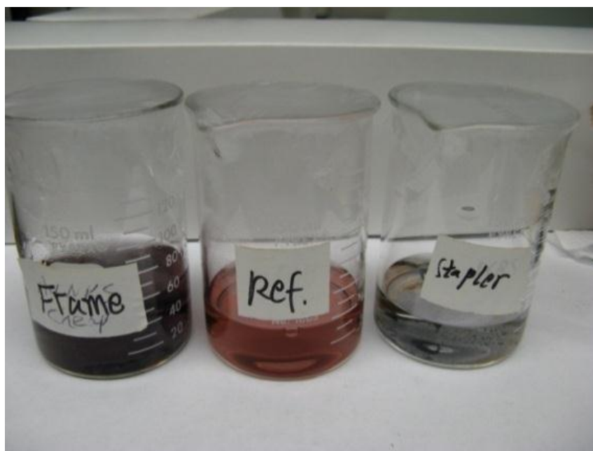
Figure 4.8. Gold nanoparticle solution degrades when in contact with polycarbonate frame (left) or stapler (right). The reference solution is shown at the center
