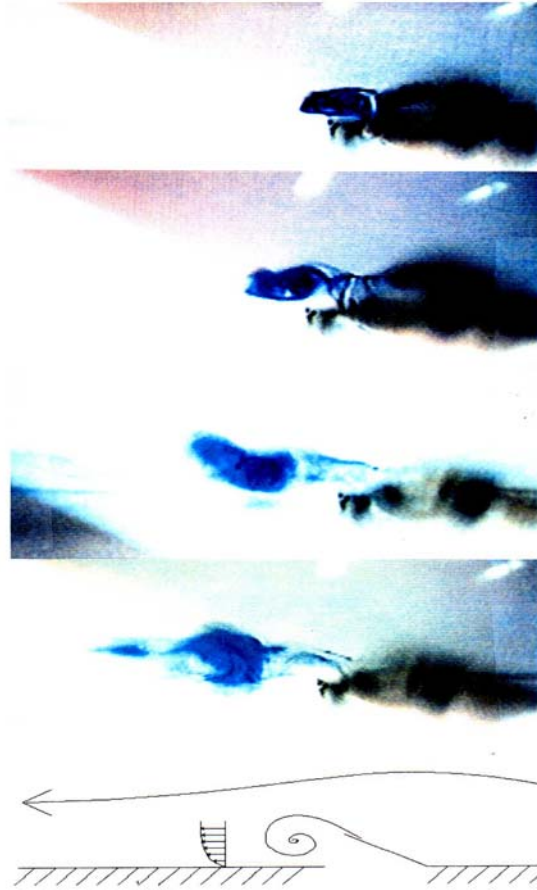
Fig. 5. Flow visualization of vortex interaction
