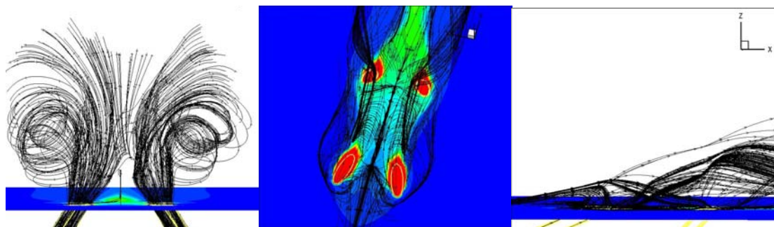
Figure 6.13 Iso-Surfaces of the aeroramp injector for various vorticity
