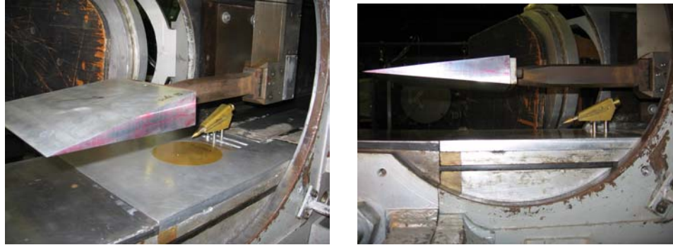
Figure 4.2. Photograph of the Test section with the Shock Generator and Concentration Probe
