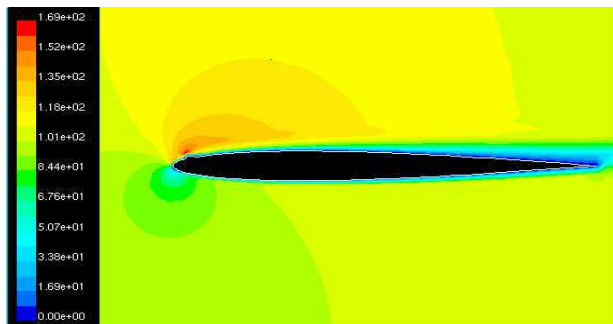
b) Onset of Boundary layer Separation
