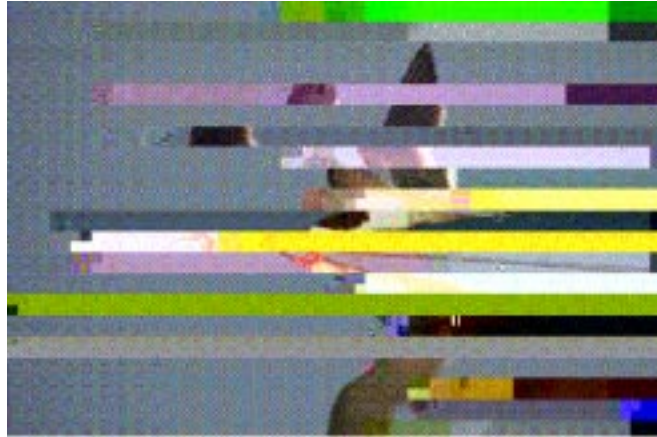
Figure 5.10: Reconstructed JPEG file from data estimated by the conventional coherent CDMA receiver ( E_b/N_o = 10 dB, N = 15 ).
