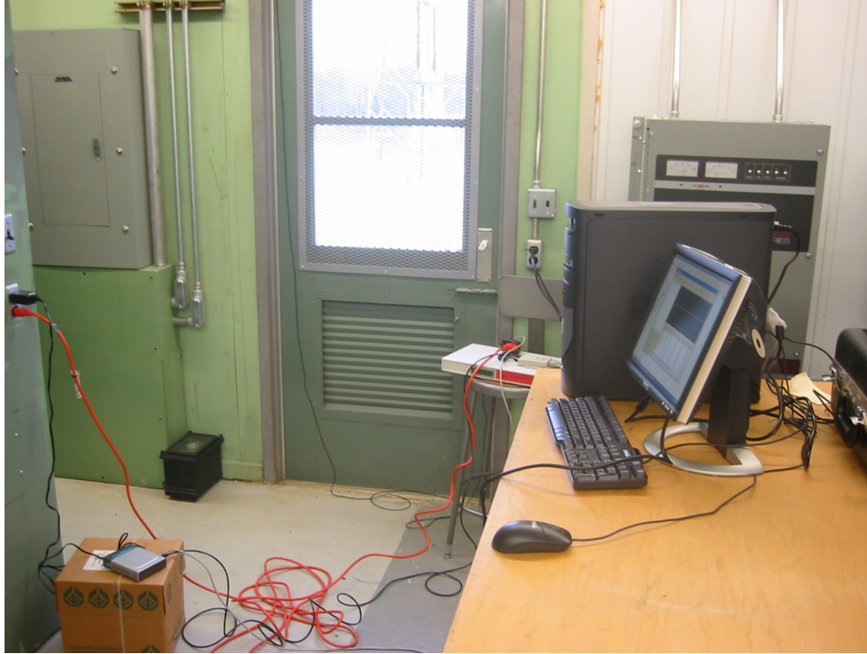
Fig 6-20. Matt Funk test setup. Right: computer & monitor, middle (white box): FDR. Left bottom corner: router.
