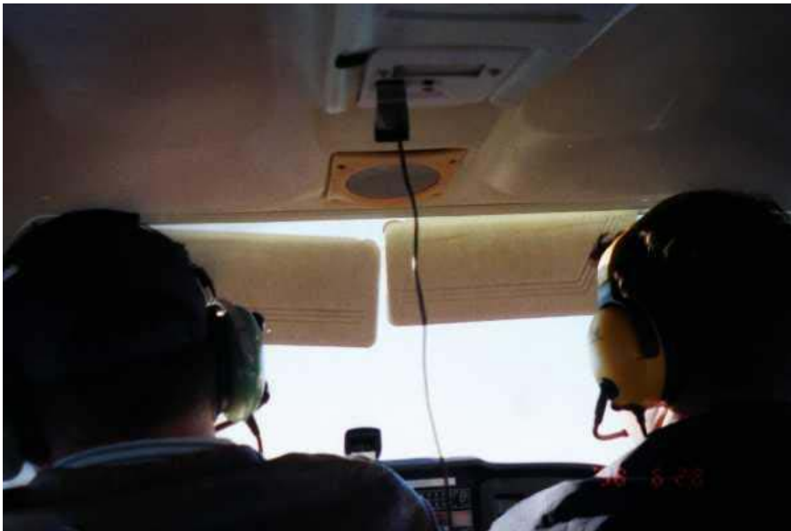
Figure 15. Miniature camera attached to cockpit ceiling.
