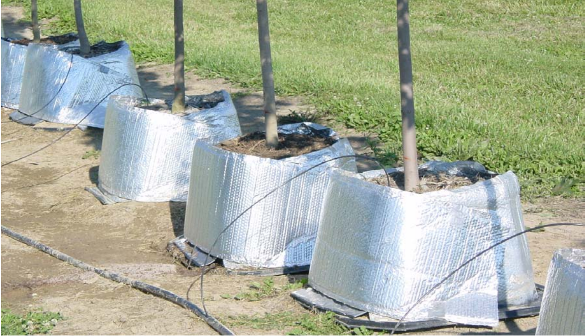
Figure A-5. Aboveground rhizotron (AGR) in nursery bed.
