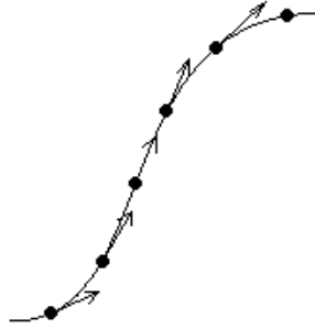
Figure 3.4 A path is approximated by a series of discrete configurations.
