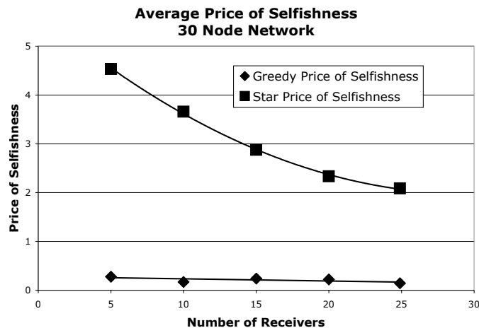
Figure 5.7: Expected price of selfishness of 30 radio network, for STAR and GREEDY routing algorithms.
