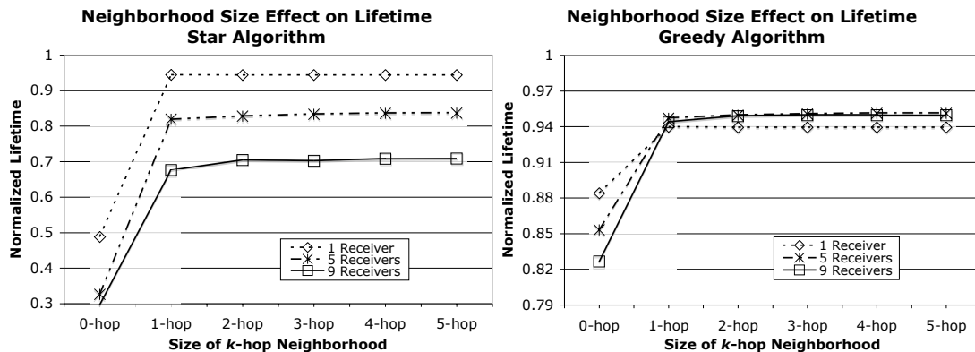
Figure 5.6: The mean normalized lifetimes of the CN for various 10 radio network k -hop neighborhoods. 0-hop neighborhoods represent the performance of the underlying routing algorithm (i.e., a “non-CN” approach). Note the differing scales of the y -axis.
