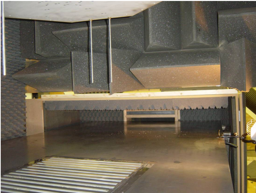
Figure 2-10 Photograph showing the acoustic enclosure around the smooth plate wall jet.
