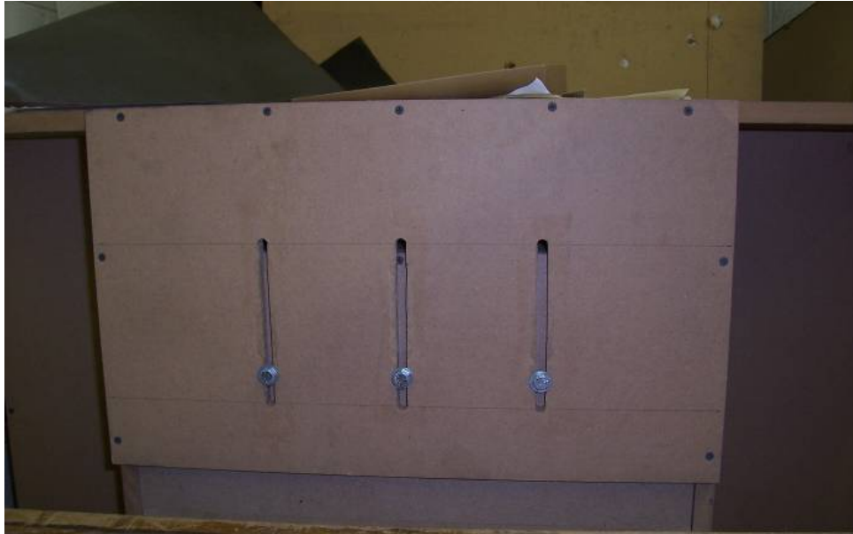
Figure 2-12 Front of preliminary settling chamber showing bolts for nozzle adjustment.
