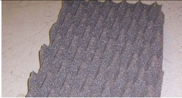
Figure 2-8 Picture of acoustic egg crate foam used to line the interior of the settling chamber. Also shown are the absorption coefficient values for the 95.25 mm thick foam.
