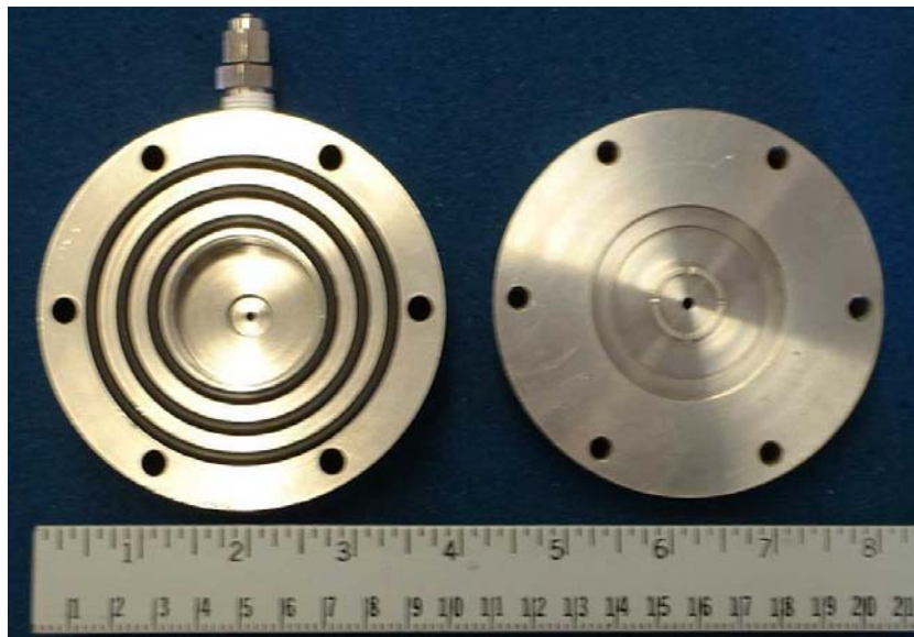
Figure 5-2. Image of the permeation cell used in this study. The left half of the cell is the feed side and contains the three gaskets used to prevent leaks. The center of the left piece is a hollow cavity. The right piece is the permeate side and hold the membrane and microporous alumina support (not shown).
