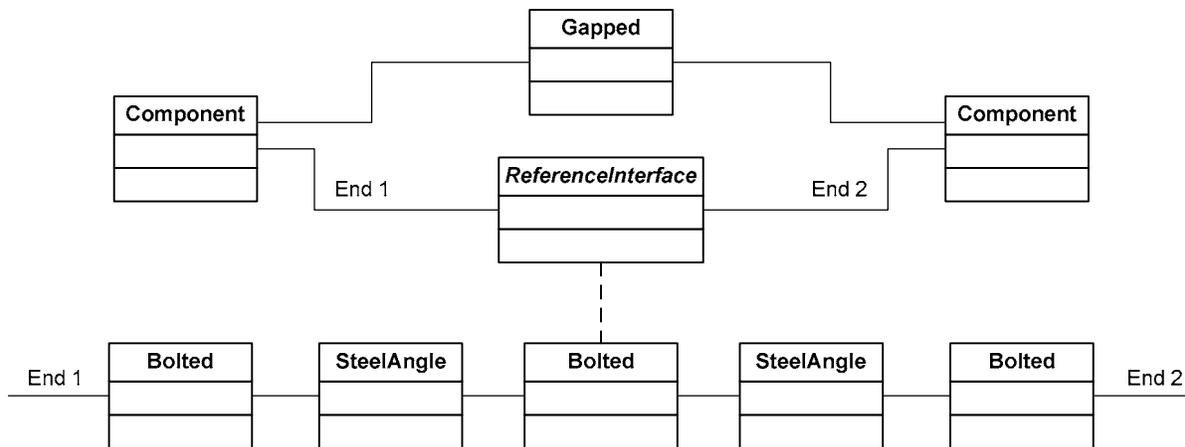
**Figure 5-3:** The Physical Interface Modeling Structure for the Selected Physical Condition
