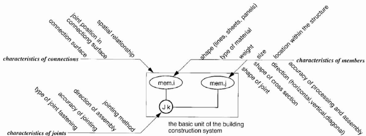
**Figure 2-4:** Characteristics of a Building Construction System (Nakajima 1998, with permission from Blackwell Publishing)
