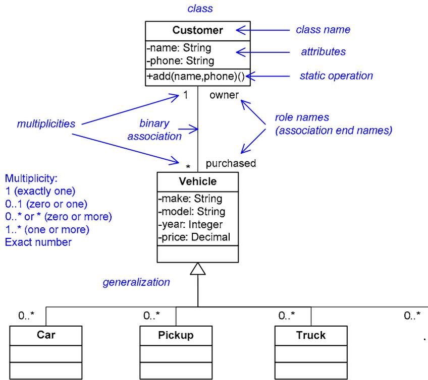
**Figure 2-10:** An Example of a Class Diagram
