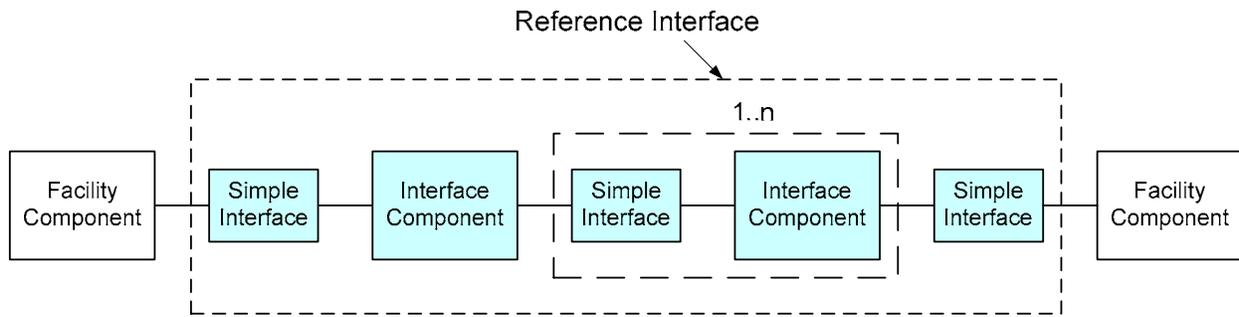
**Figure 4-12:** The Compound Type of Reference Interface
