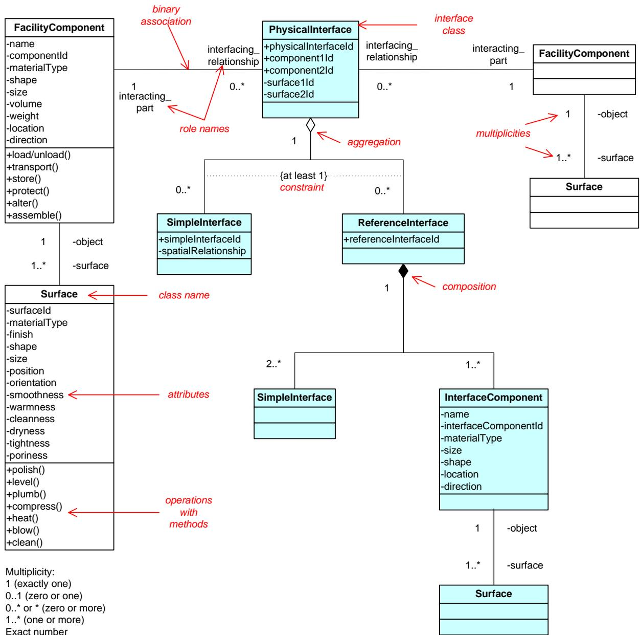
**Figure 4-10:** Data Dependency Between Physical Interface Objects and Facility Components
