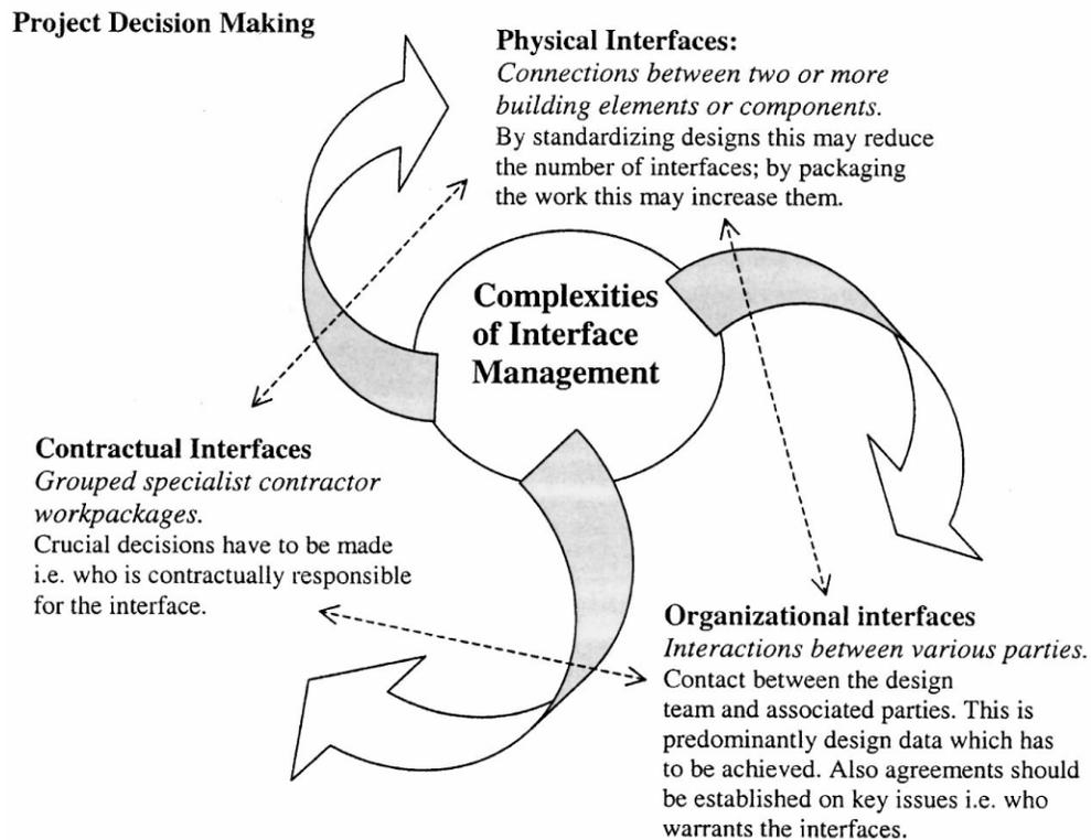
**Figure 2-1:** Complexities of IM (Pavitt and Gibb 2003, with permission from ASCE)
