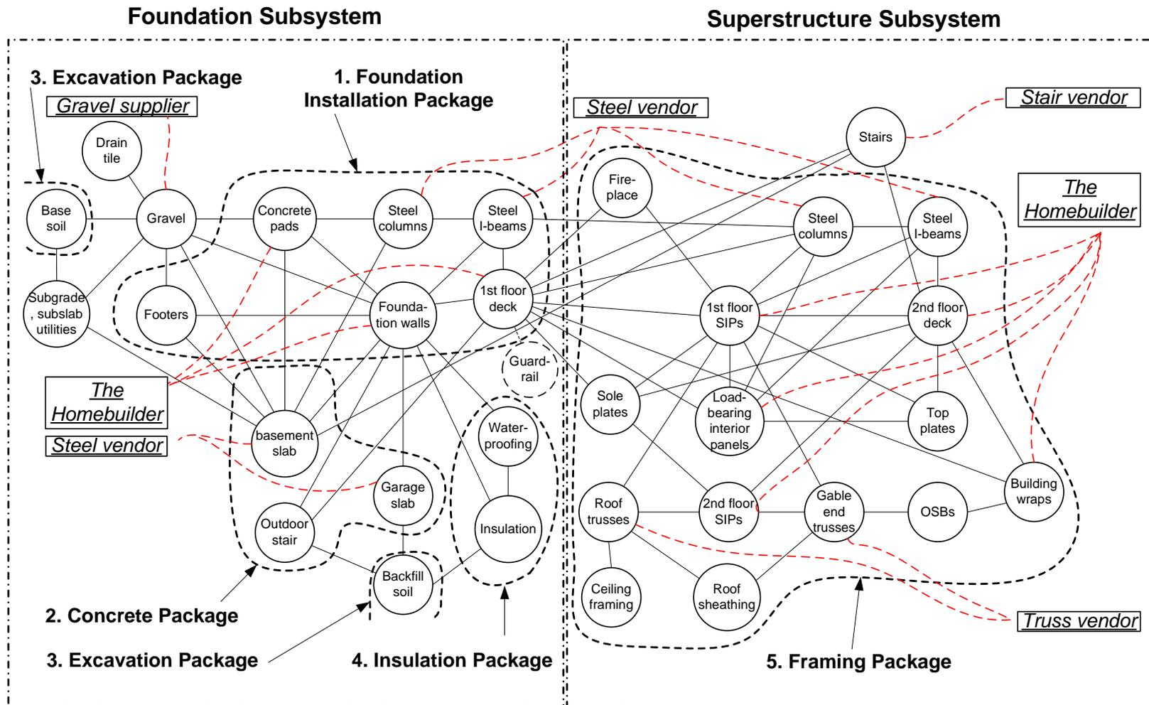
Figure 5-12: Overall Structure of Foundation and Superstructure Subsystems
