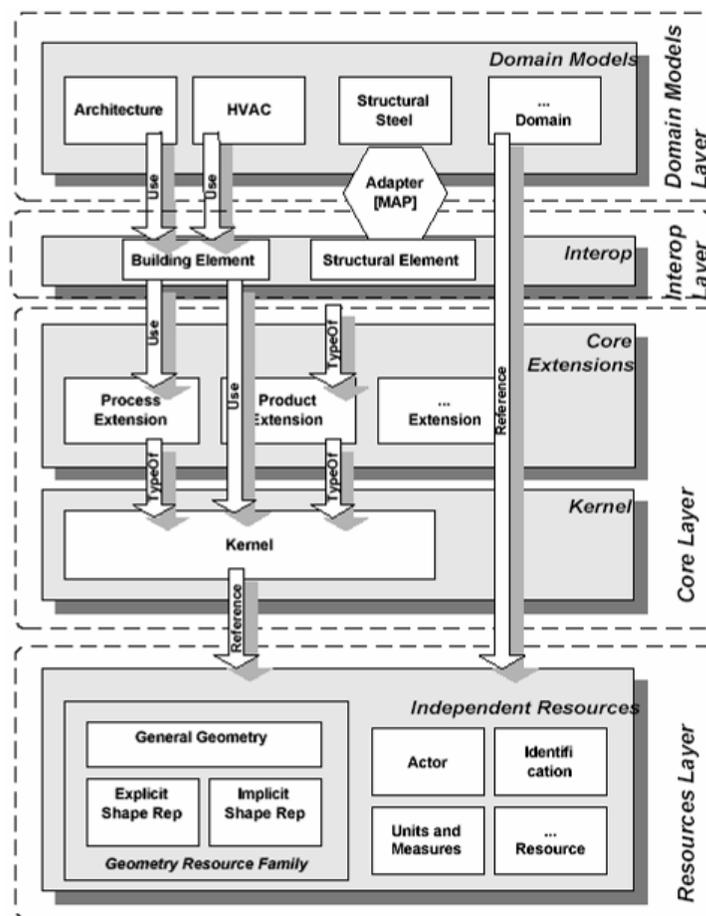
**Figure 2-8:** IFC Object Model Architecture (Wix and Liebich 1997, with permission from CIB)
