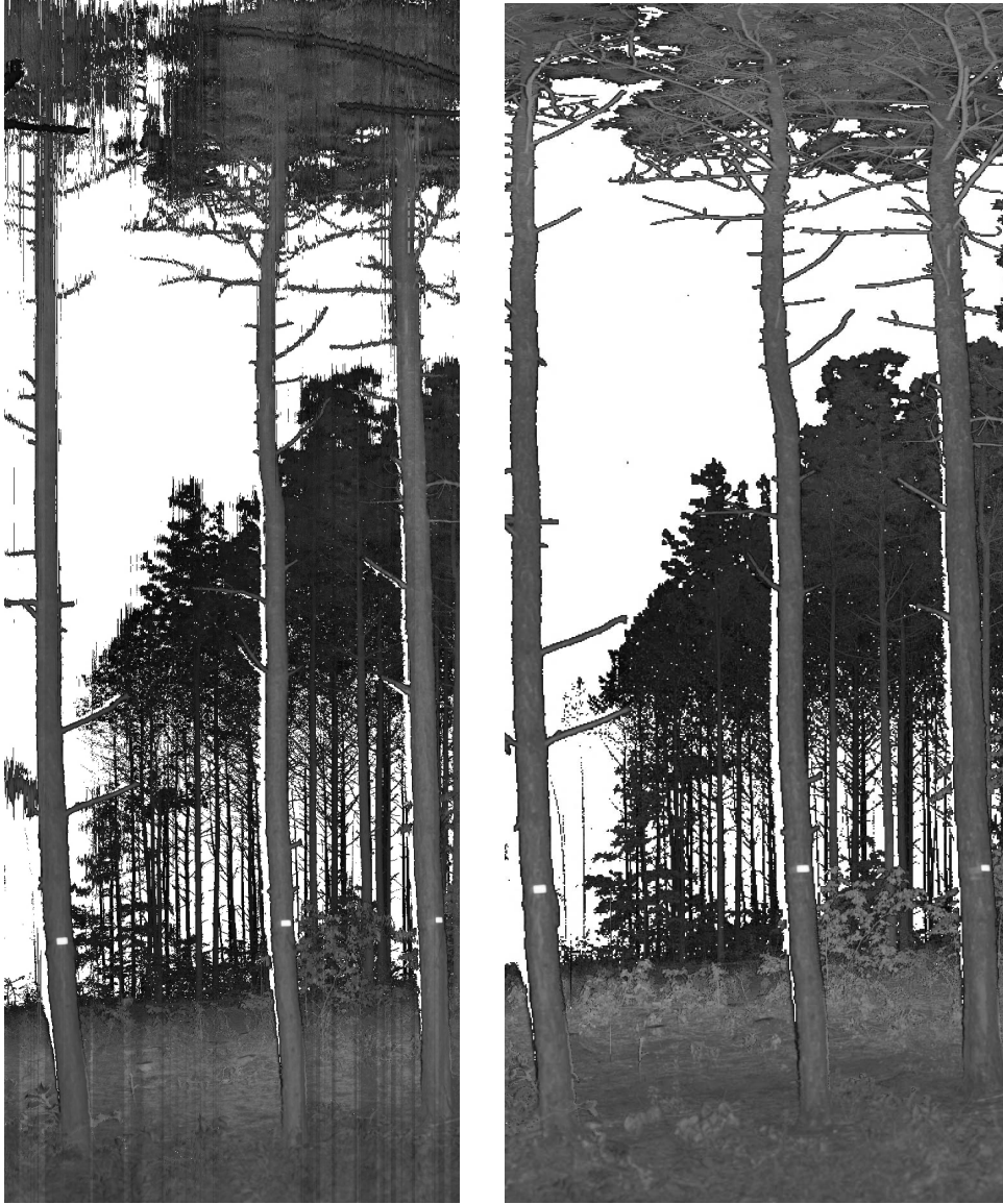
Figure 3.2. Scan C (Figure 3.1) laser pulse return intensity from three target trees in the foreground and a forest edge in the scene background. Tree movement due to light winds is indicated by vertical striae, especially high in the canopy where movement is greatest (left). Under calm conditions distortions are less apparent (right).
