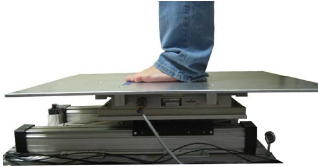
Figure 4.1 – Experimental set-up of the pneumatic instrumented moving platform. The platform translated 0 to 0.15 m forward and 0 to 0.25 m backward over 360 ms. A force platform was integrated with the moving platform and used to quantify balance. Photo by author, 2009.
