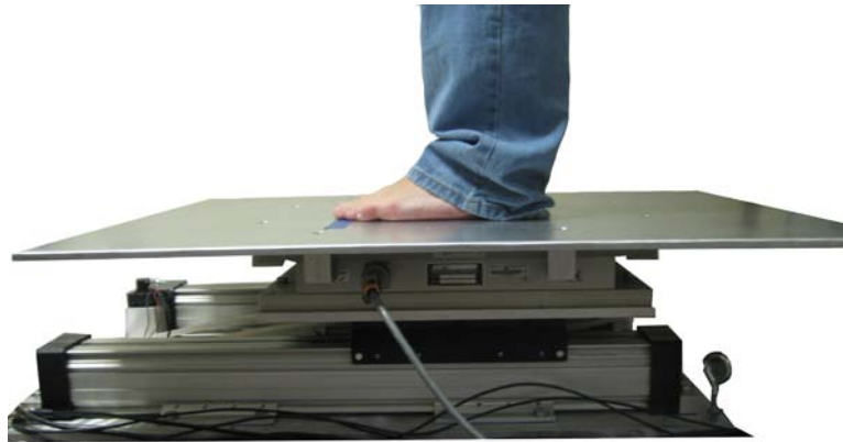
Figure 3.1 – A pneumatic instrumented moving platform was used for all testing and training sessions. A force platform was mounted on the platform and used to quantify balance. Photo by author, 2009.
