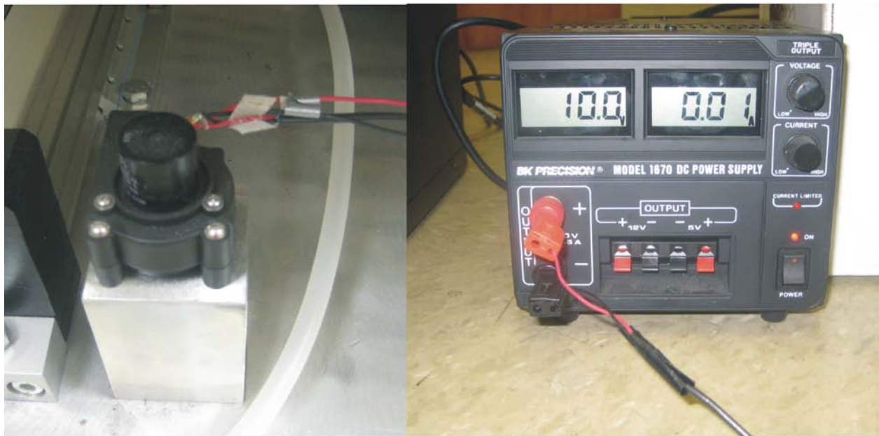
Figure A.6 – Left side shows close-up of linear potentiometer. Right side shows the power supply set to 10 V. Photo by author, 2009.
