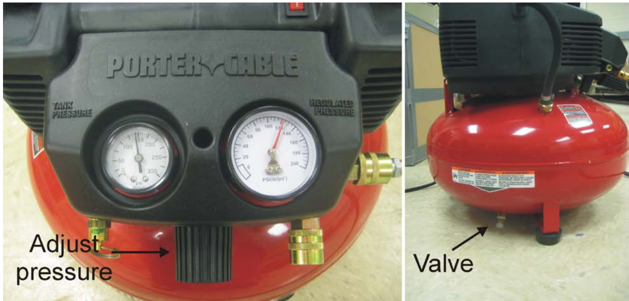
Figure A.5 – Air compressor used to run the moving platform. The knob is used to adjust the pressure to 120 psi. The valve must be closed prior to filling the tank with air. Photo by author, 2009.
