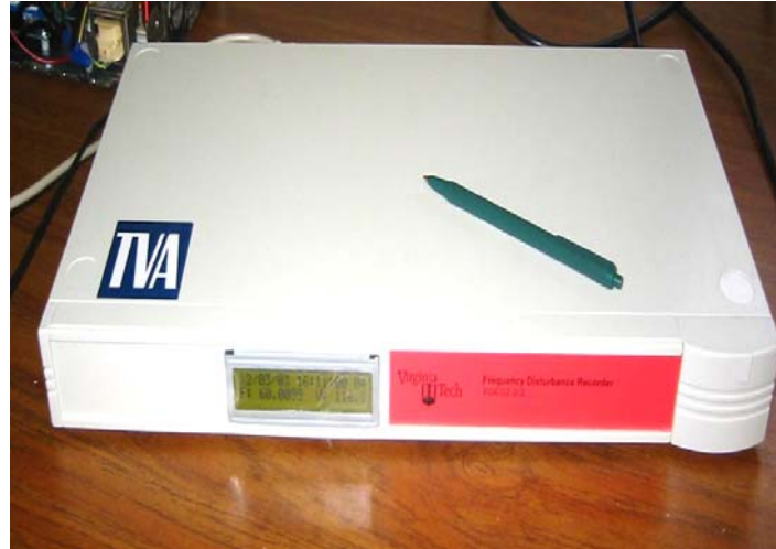
Fig. 5-22. Frequency disturbance recorder (FDR) outline
