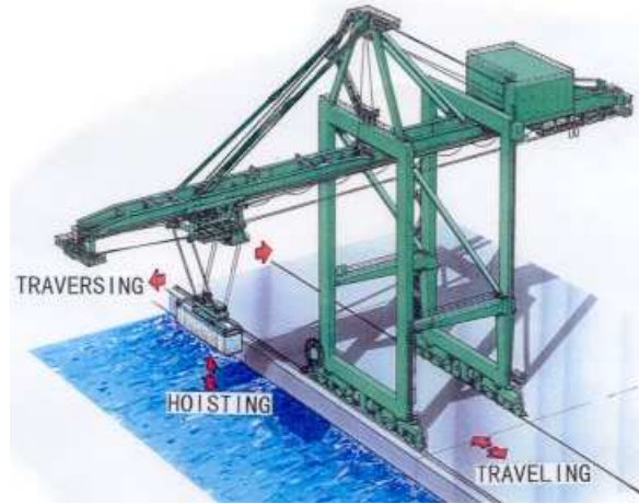
Figure 1.1: Typical quay-side container crane.
