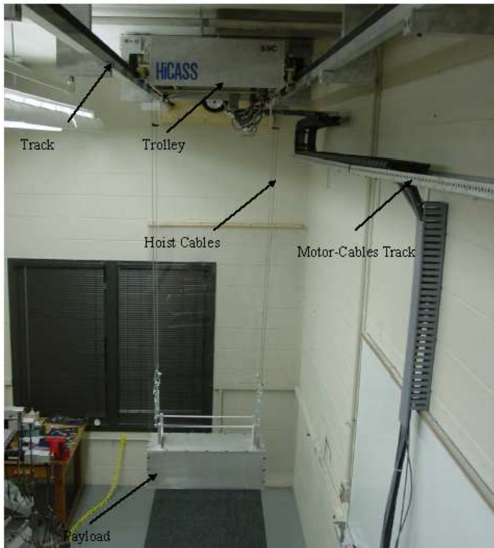
Figure 4.1: A 1:10 scale model of a 65-ton quay-side container crane.
