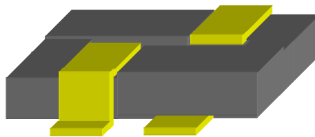
Figure 3.37 The low profile twisted-core coupled-inductor
