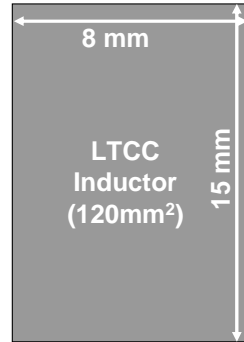
Figure 4.52 One w and l dimension case of the LTCC coupled inductor structure 2 for the footprint 120\text{mm}^2 ( w=8\text{mm} , l=15\text{mm} )
