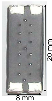
Figure 4.69 The final two-phase LTCC integrated coupled-inductor structure 2 prototype ( w_1=2\text{mm} , w_2=1\text{mm} , w_s=1.5\text{mm} , t_1=0.7\text{mm} , t_s=2\text{mm} and l=20\text{mm} )
