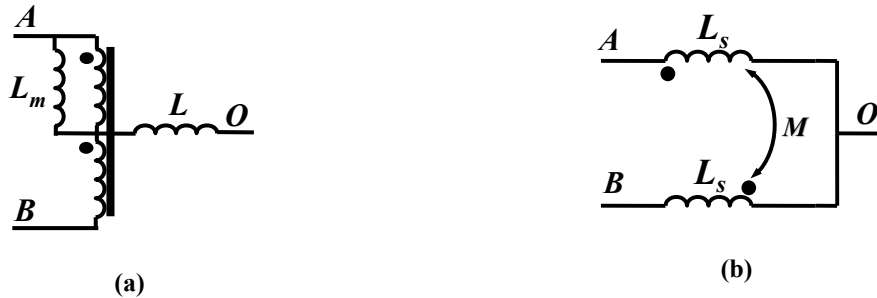
Figure 1.36 Two transformation of the two types of coupled-inductors (a) Representation of Advanced Energy’s two-phase coupled-inductor (b) Representation of P. Wong and C. Sullivan’s two-phase coupled-inductor
