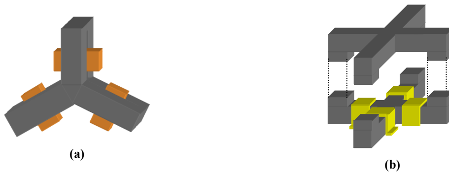
Figure 1.39 The symmetric three-phase and four-phase coupled-inductor structures (a) The three-phase coupled-inductor structure (b) The four-phase coupled-inductor structure
