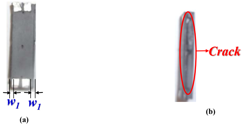
Figure 4.67 The LTCC integrated coupled-inductor 2 prototype when w_1=1\text{mm} ( w_2=1\text{mm} , w_s=1.5\text{mm} , t_1=0.7\text{mm} , t_s=2\text{mm} and l=20\text{mm} ) (a) the top view (b) the side view
