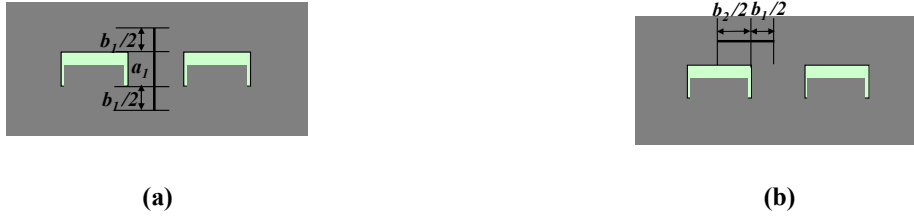
Figure A2.25 The magnetic core 1 reluctance R_{core1} and the magnetic core 2 reluctance R_{core2} (a) The magnetic core 1 reluctance R_{core1} (b) the magnetic core 2 reluctance R_{core2}
