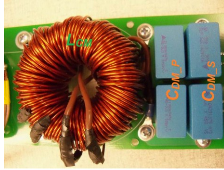
Fig. 3.27: AC CM choke and AC DM capacitors
