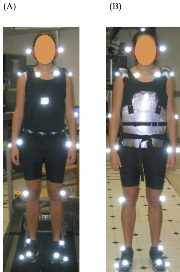
Figure 3. 1. Subject with reflective markers (A) unloaded walking and (B) loaded walking.
