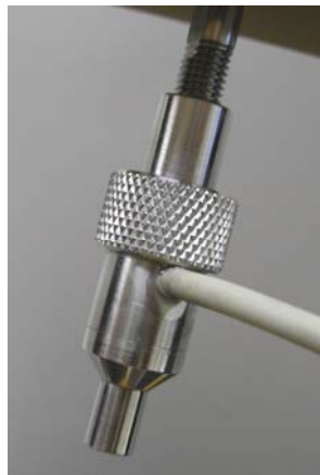
Figure A-7. Integrated load cell and anvil from Custom Design and Fabrication.
