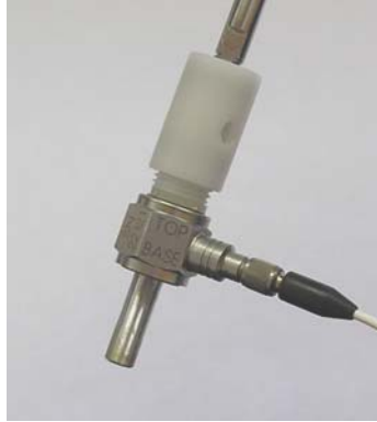
Figure A-2. PCB load cell with shock adapter and aluminum anvil attachment.
