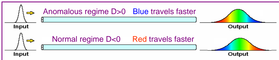
Figure 3-2. Illustration of Pulse Broadening by Group-Velocity Dispersion
