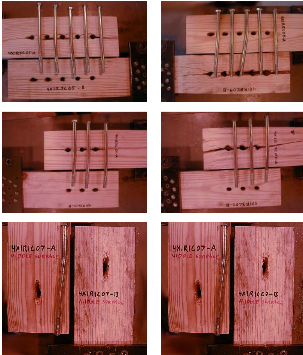
Figure 10.7: Yielded bolts and their corresponding location within the joint after cyclic tests (from Anderson (2001)). The top row shows two 5-bolt joints predicted to yield in Mode IV, but only Mode III and some Mode II yield can be observed. Middle row depicts two 3-Bolt joints predicted to yield in Mode IV. Again only Mode III and Mode II can be observed. The bottom row shows two single-bolt joints exhibiting the predicted Mode IV yield.
