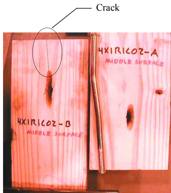
Figure 10.11: Failure mode in single-bolt Mode IV specimens was primarily wood crushing. Still, at larger displacement brittle failure was frequently detected (from Anderson (2001)).
