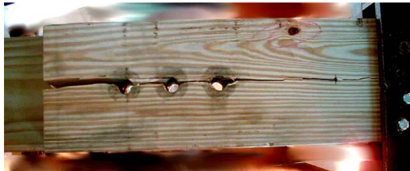
Figure 10.9: Failure initiated by a single crack due to tension perpendicular-to-grain stresses. Note that the crack does not run through the centerline of the joint (from Anderson (2001)).
