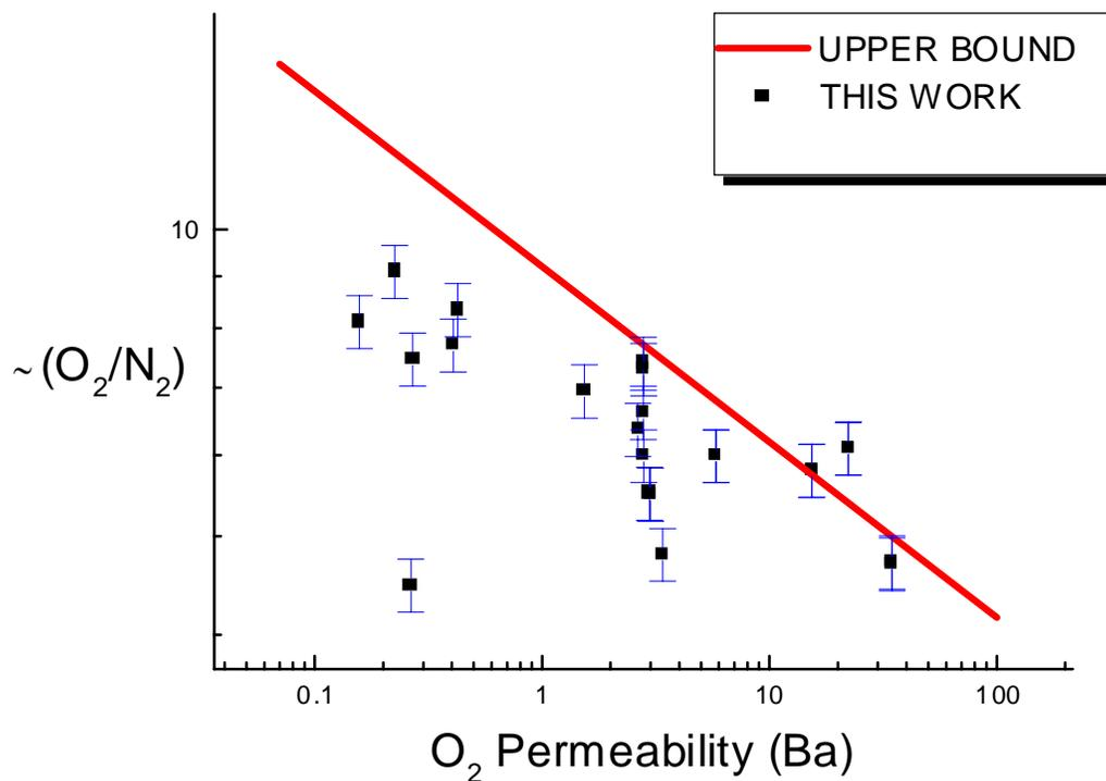
\*error bars for  $\alpha(O_2/N_2)$  values in blue ( $\pm 6\%$ ); error bars for O<sub>2</sub> permeability values were omitted due to being indistinguishable from the data points on this scale ( $\pm 3\%$ )
