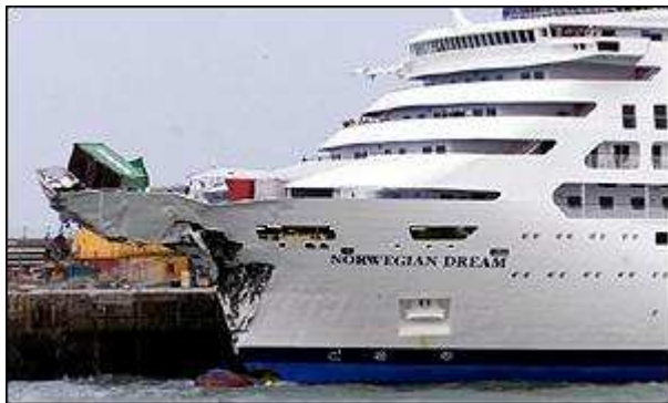
Figure 2-9 Bow Damage to Norwegian Dream
