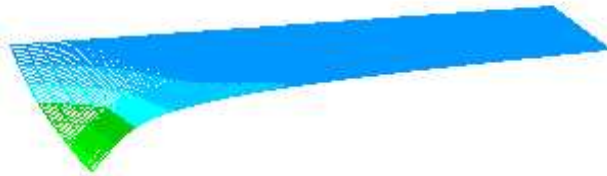
Figure 5-71 Test Case 4 FEA Plate Mesh Deflection at 0.35 Seconds
