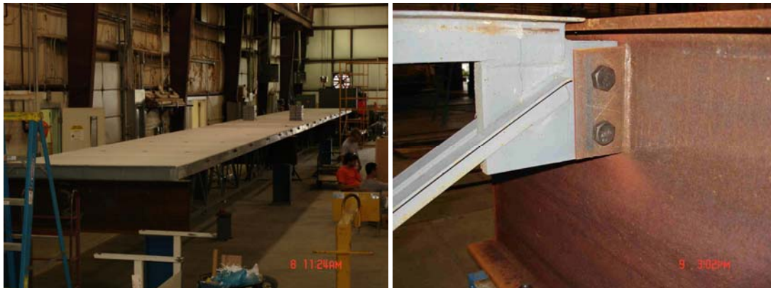
Figure 2.3: Shear-Connected Joist Footbridge Specimen
