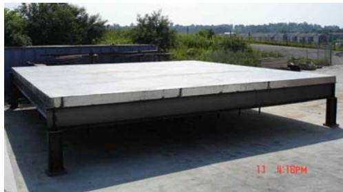
Figure 2.1: Long Span Composite Slab Laboratory Specimen
