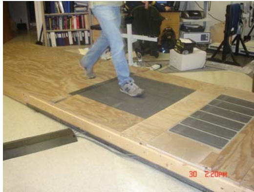
Figure 2.27: Footstep Force Measurement
