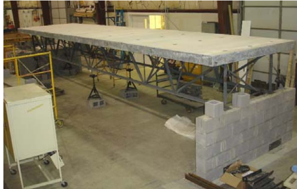
Figure 2.2: Shear Connected Joist Footbridge Laboratory Specimen
