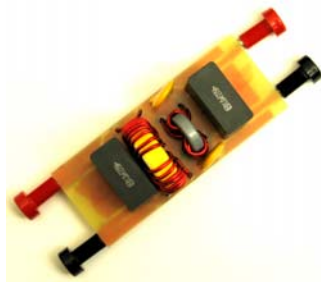
Figure 4.9. Filter prototype for the 4-channel PFC with phase shedding and phase angle control.
