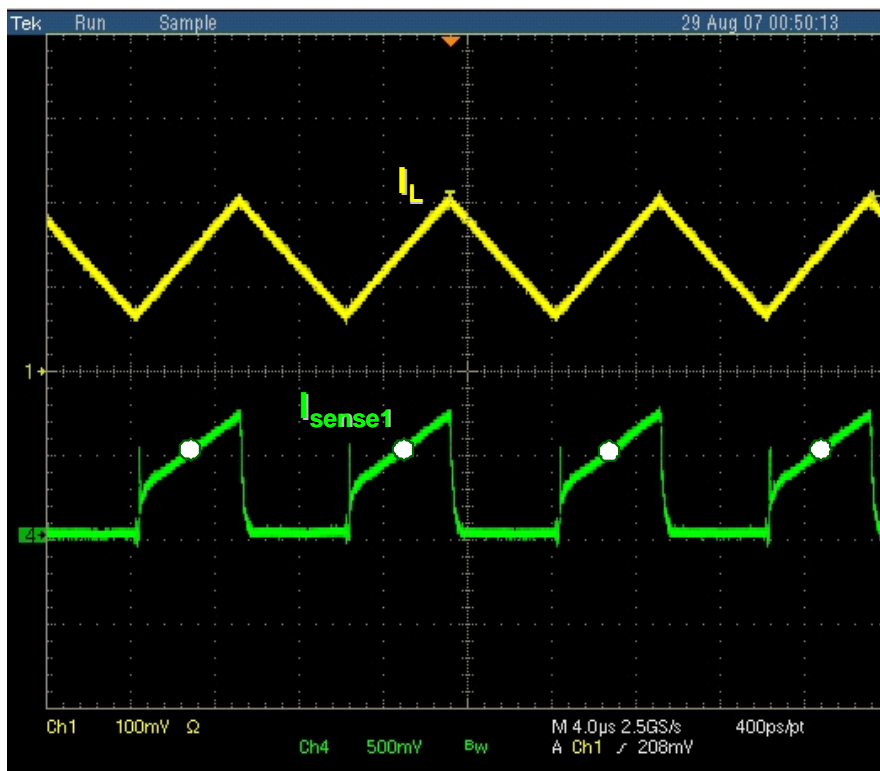
Figure 3.19. Experimental current sensing waveform.
