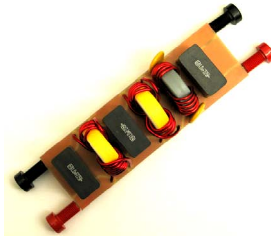
Figure 2.12. EMI filter prototype for the benchmark PFC.
