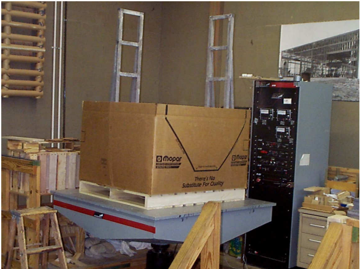
Figure 17. Vibration test set-up for unit load validation test
