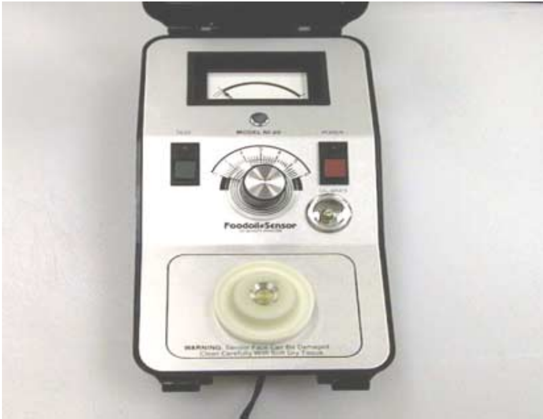
Figure 6.2 FoodOil Sensor model NI-20 for measuring dielectric constant.
