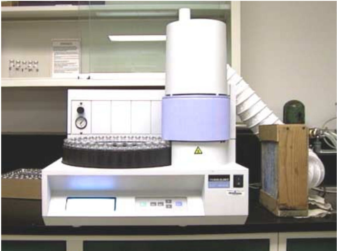
Figure 6.3 Chemosensory system model QMB-6 connected to HS40 XL auto sampler.
