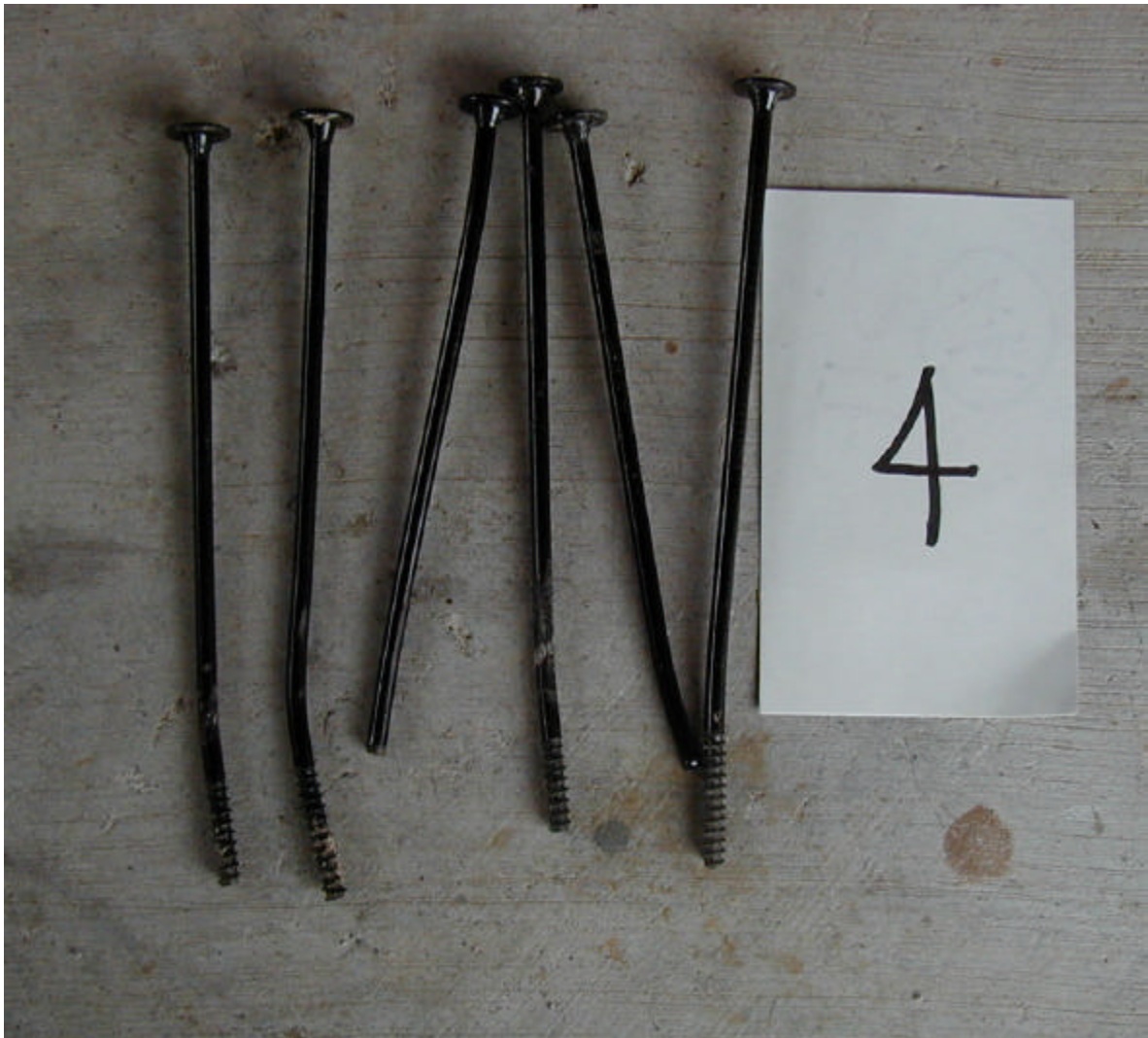
Figure B.1. Examples of bent and broken screws extracted from Assembly 4 after failure.
