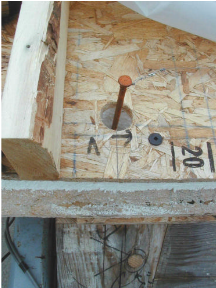
Figure 3.14. Example of pin driven into timber and 1-1/2 in. (38 mm) hole drilled through SIP. Pin was utilized for diagonal displacements for use with shear deformation determinations.
