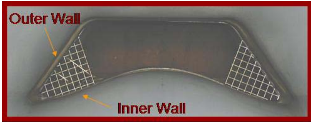
Figure 3.11 Pressure Loss Grids used to Simulate Angle of Attack (Screen Material)
