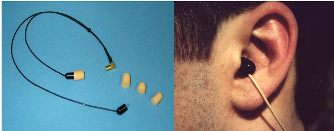
Figure 1. Communications earplug (CEP) assembly (left) and as worn in the ear (right).
