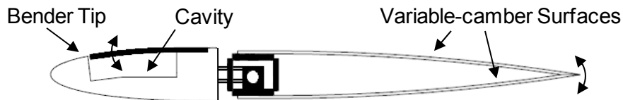
Figure 7.2: Illustration of the variable-camber airfoil with flow control feature.
